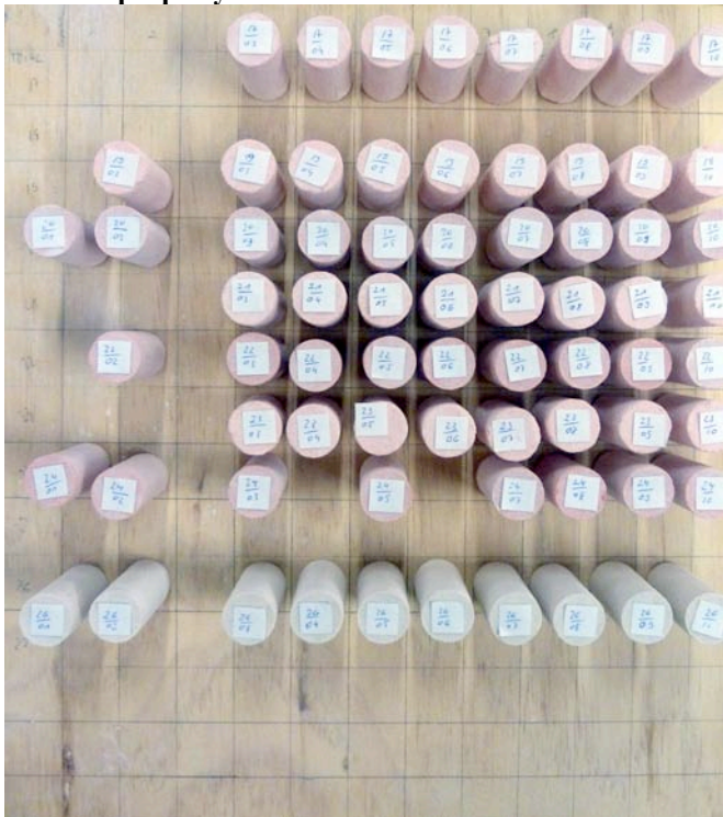
Fig. 2 Samples of prototype cylinders developed using additive manufacturing processes in preparation for material property tests.
