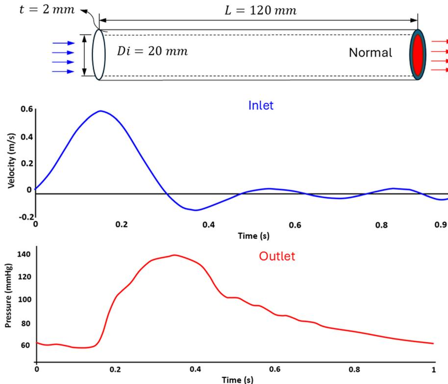
**Fig. 1 The computational domain and the boundary conditions for the healthy artery (adapted from Ref. [4])**
