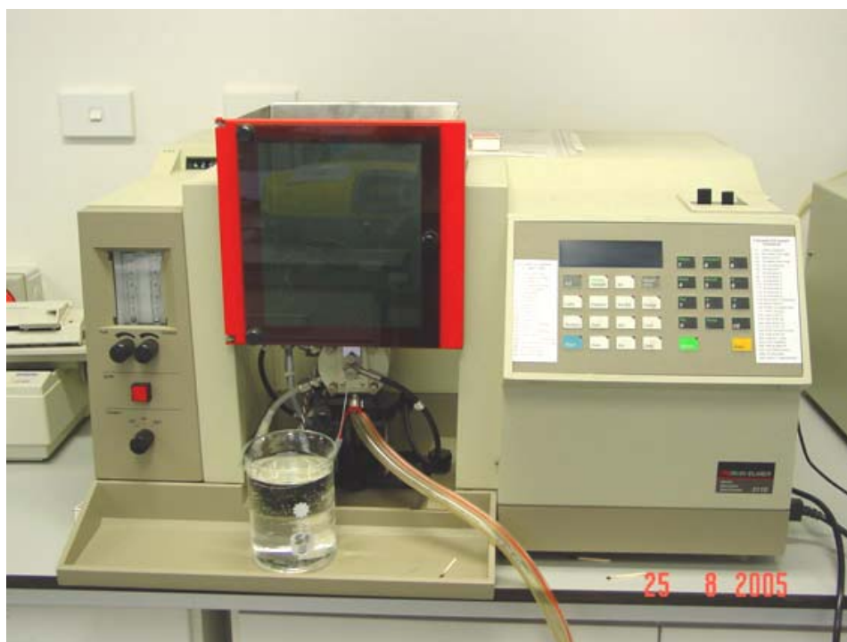
Figure 2.1 The Perkin-Elmer 3110 flame atomic absorption spectrometer used for all metal analysis conducted at AUT
