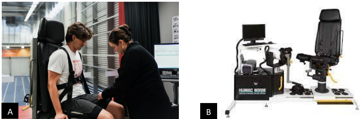
Figure 2. Participant strapped into the seat of the Humac Norm machine(A) and an image of the full apparatus(B).
