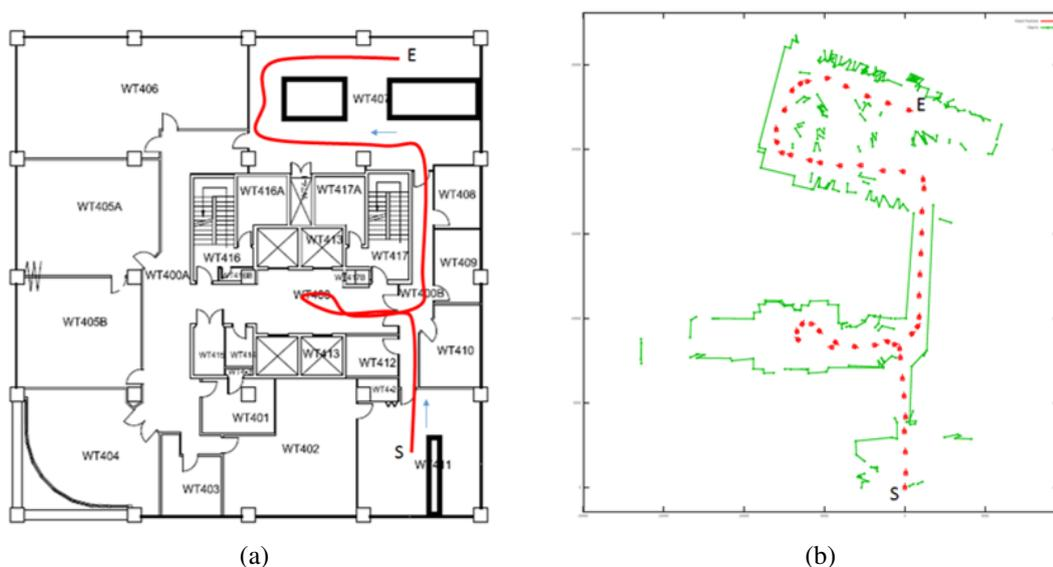
Figure 3.10: (a) The environment and the path taken. (b) The trace map generated.
