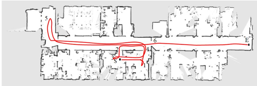
Figure 4.29: The environment and Albot1's path for Experiment 13.
