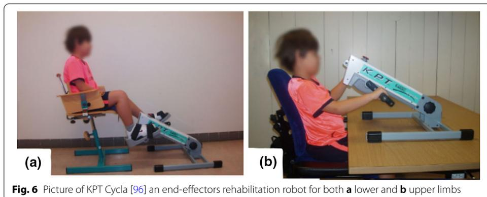
**Fig. 6** Picture of KPT Cyclia [96] an end-effectors rehabilitation robot for both **a** lower and **b** upper limbs
