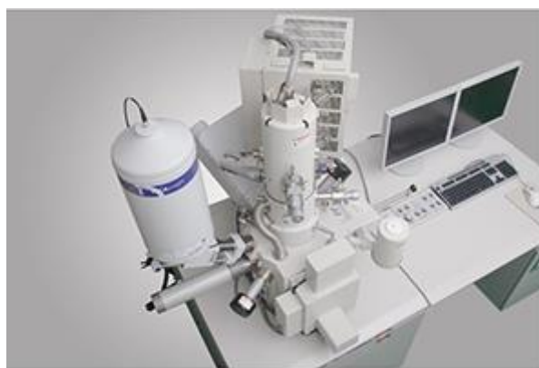
Fig 3. 3 Hitachi SU-70 scanning electron microscope (SEM) instrument
