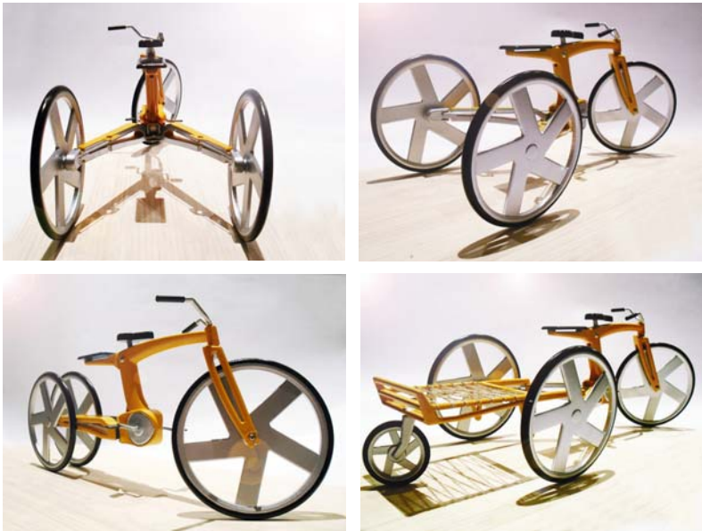
Fig 22. -25. Semi working scale model rapid prototype.
