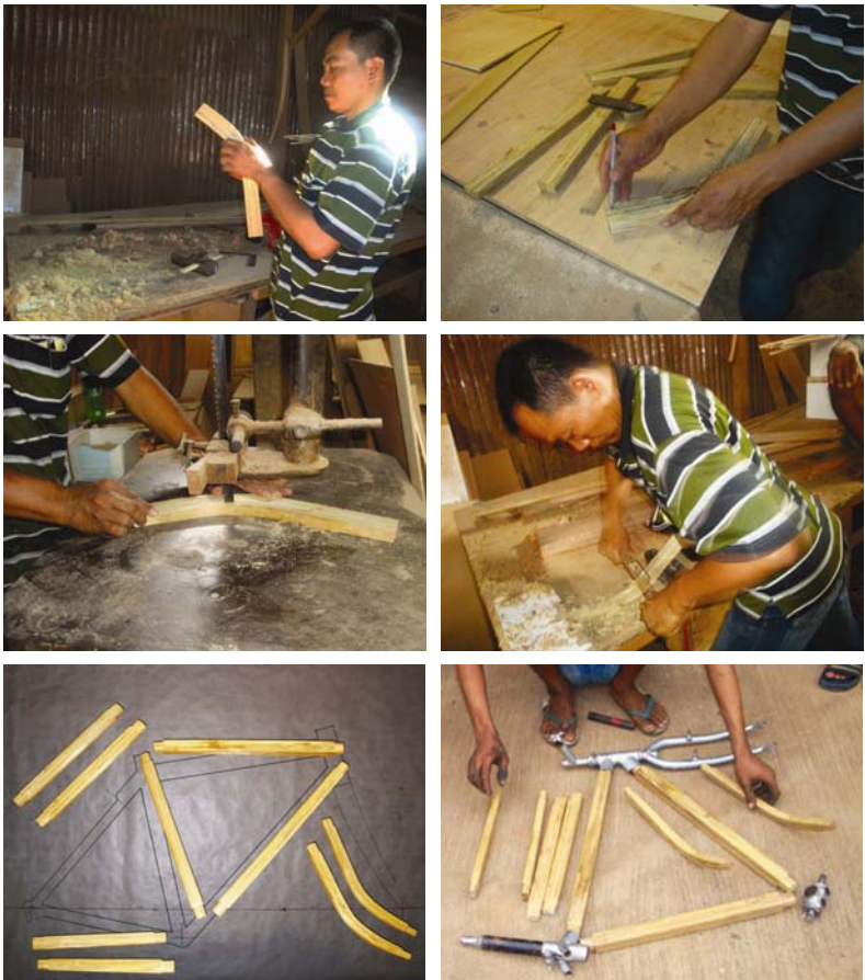
Fig 33. Construction processes of bamboo laminated frame no.1
