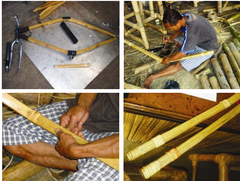
Fig 36. Construction processes of bamboo laminated frame no.2
