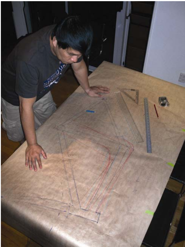
Fig 39. Producing the full scale of Greencycle frame pattern.
