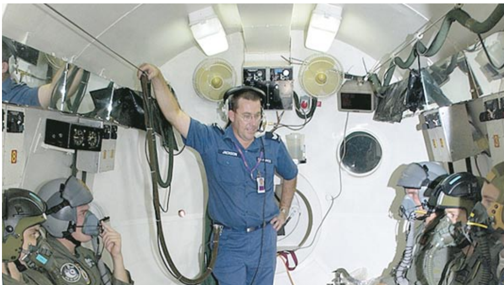
Figure 2. Example of the inside of hypobaric chamber being used for pilot hypoxic training ( http://www.defence.gov.au )
