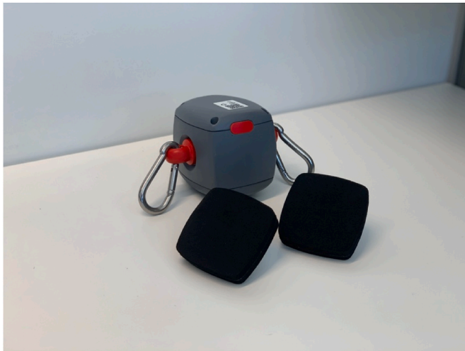
Fig. 3. Strain gauge, including carabiners and push plates.
