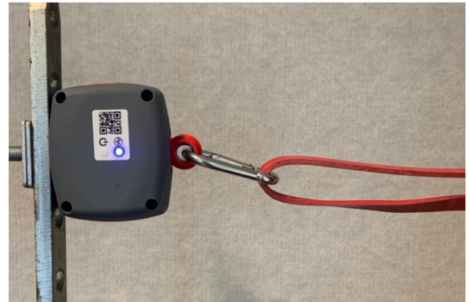
Fig. 4. Strain gauge affixed to a rack and the EBR affixed to the strain gauge.
