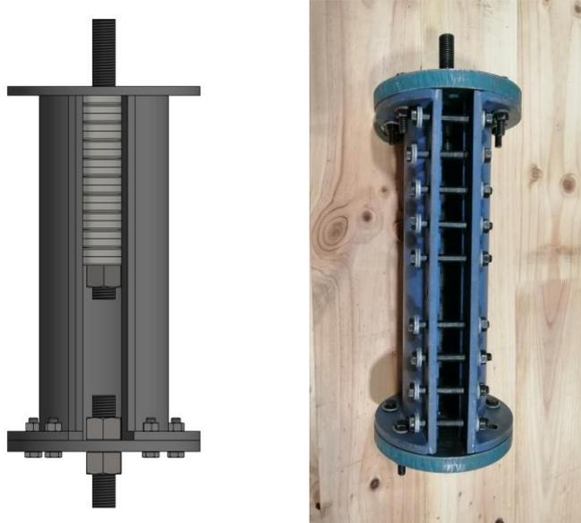
Figure 3-10 The utilized sleeve for testing of disk springs
