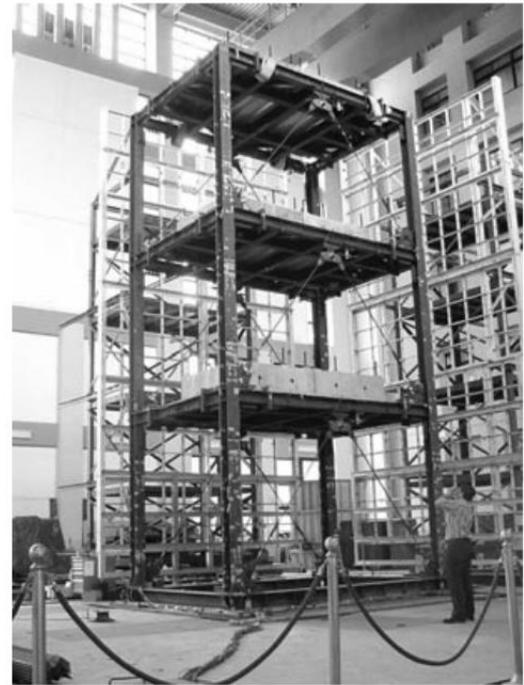
Figure 1-3 Components of the first introduced rotational Friction damper[23] (Left); Implementation of the rotational friction damper in a three-story steel building for shake table test[28] (Right)
