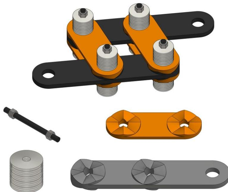
Figure 3-1 The SC-RF damper and its components, including cap and middle plates, disk springs, high strength bolt or rod
