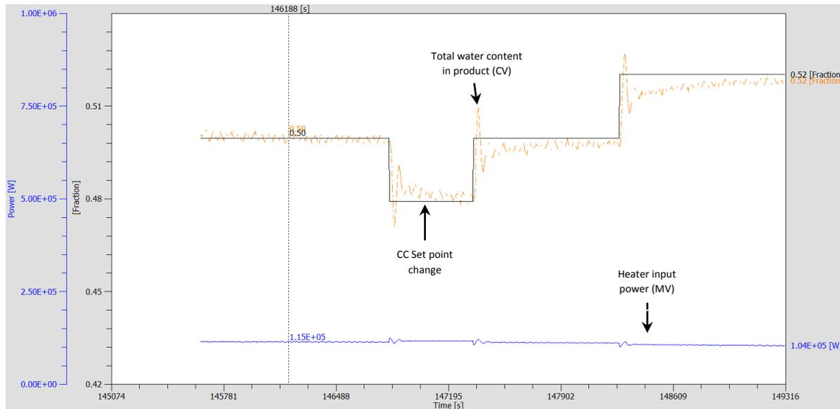
Figure 7. Snapshot of dynamic model control performance
