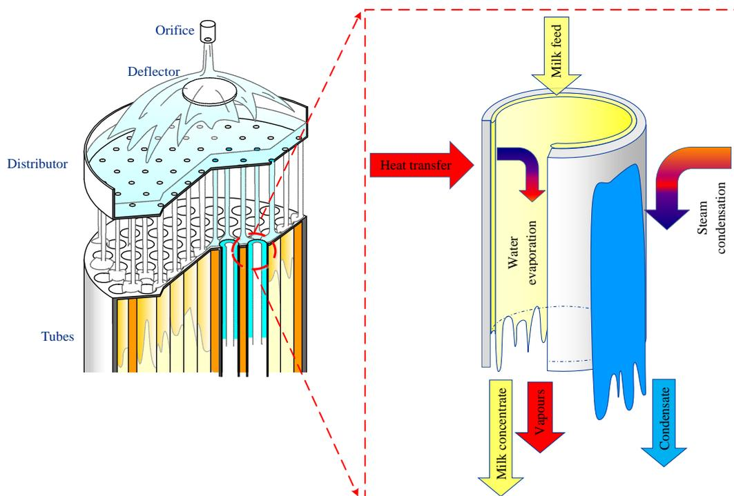
**Figure 4.** Basic principle of falling film evaporation
