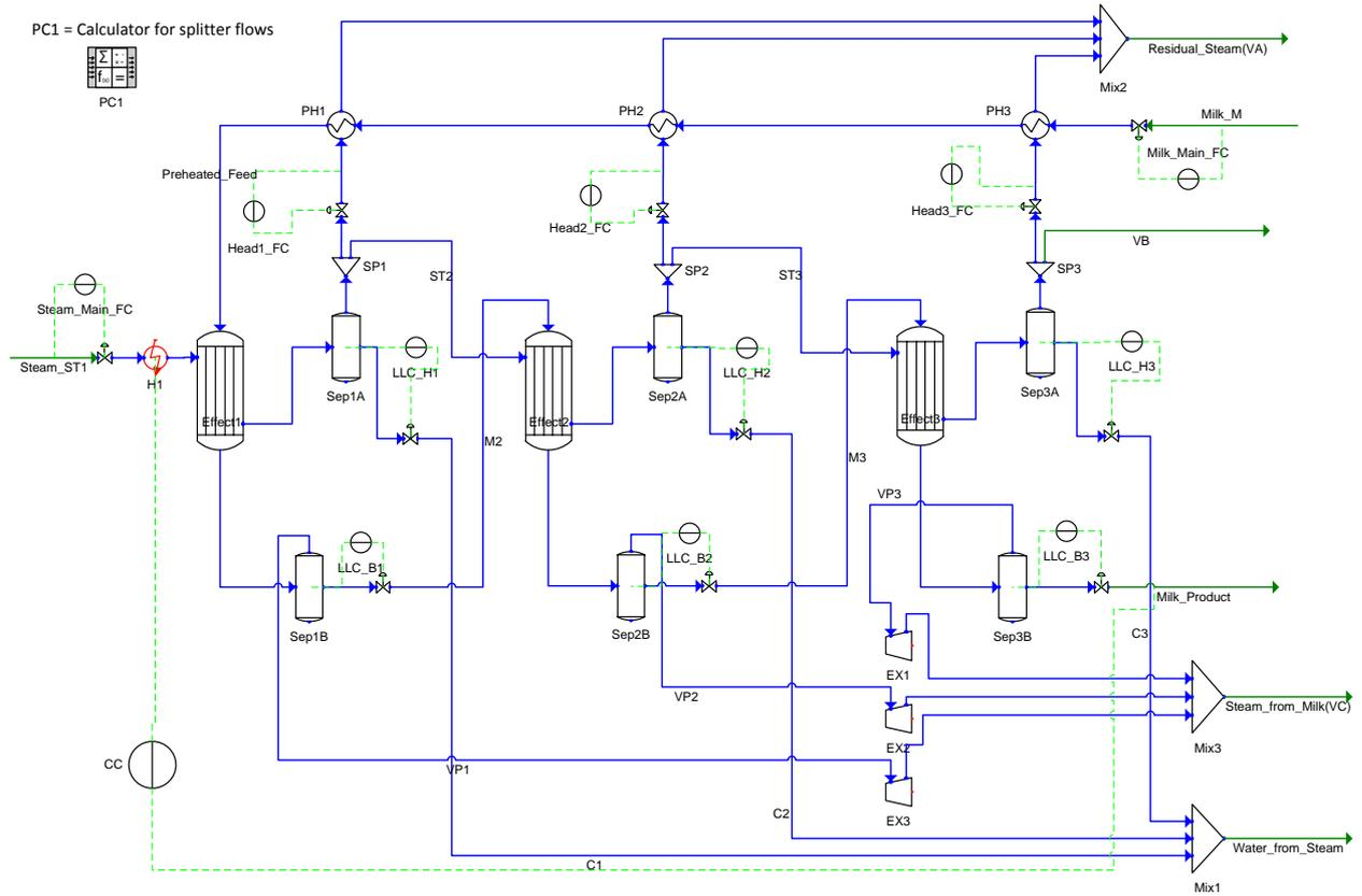
Figure 6. Multi-effect falling film evaporator dynamic state model
