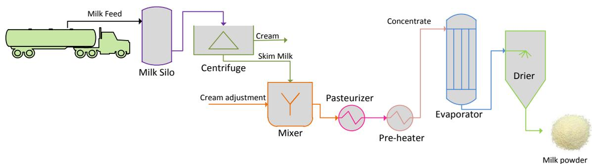
Figure 3. Milk powder manufacturing process schematic
