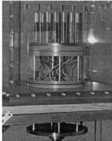
Figure 3-1 Monopole antenna array for tomography Imaging, Meany P.M et al. [44]
