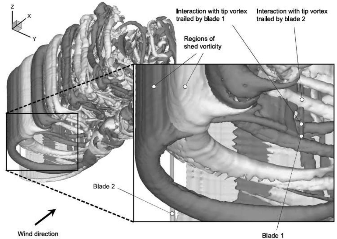
(b) Interaction between blade 1 and its own trailed vortex and the tip vortex trailed by blade 2.
