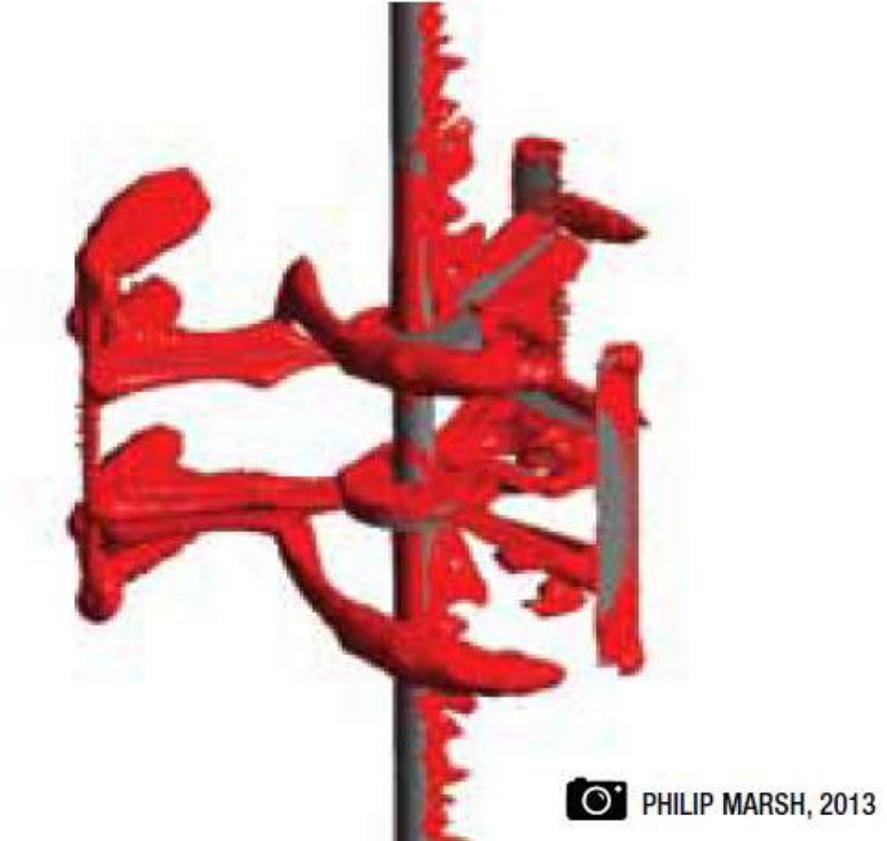
Figure 10 (left): Flow velocity  $\bar{w}$  (m/s) for the 3D Computational Fluid Dynamics model with appendages at  $\lambda$  of 2.
