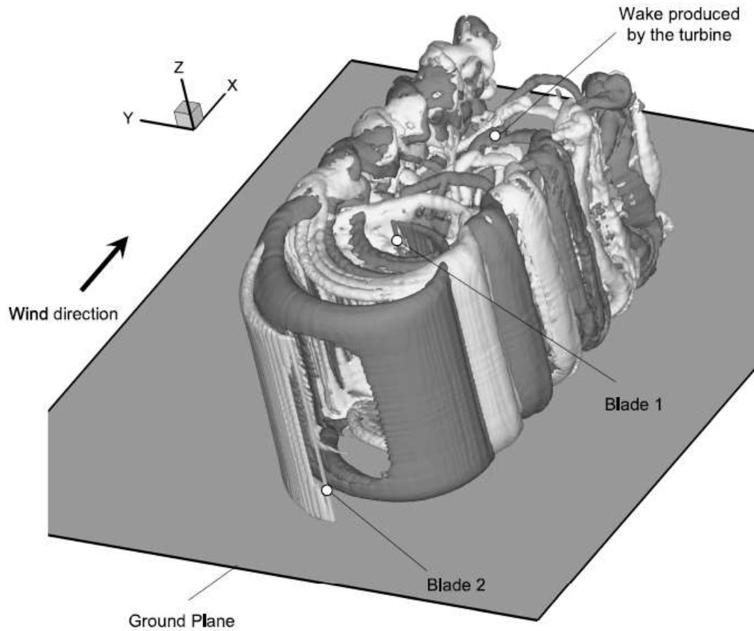
(a) Propagating wake produced by the turbine.
