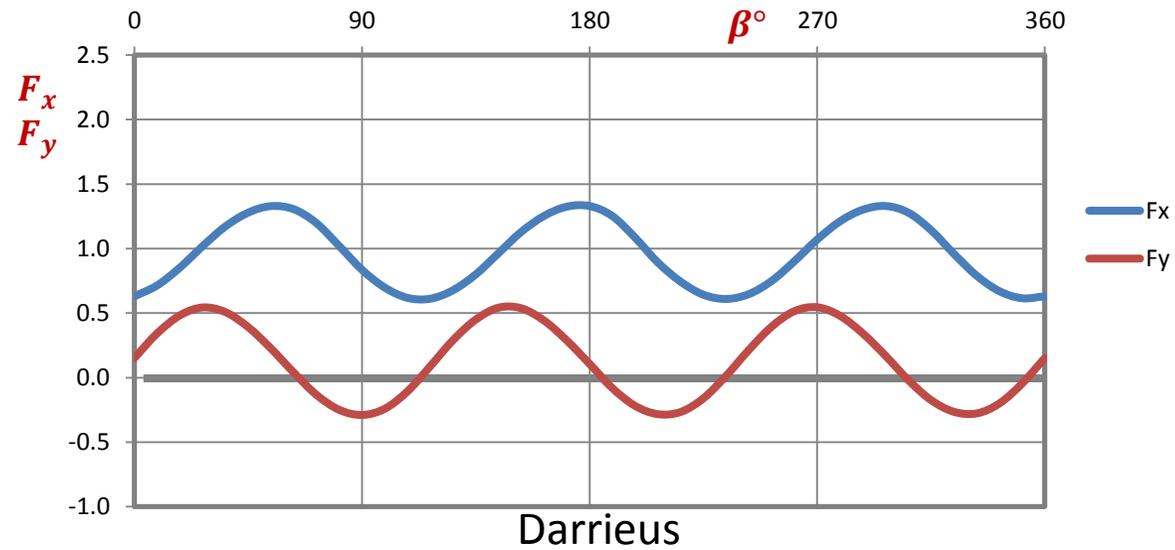
**Tower Forces  $F_x$  vs  $\beta^\circ$  and  $F_y$  vs  $\beta^\circ$  at  $\lambda = 3.6$**
