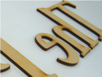
Figure 2:4 Laser-cut 3mm MDF board ready to use as a debossing effect.
