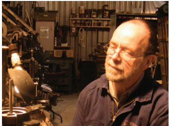
Figure 2:3 TATATM volunteer Terry Foster preparing slugs of lead type on an Intertype casting machine.
