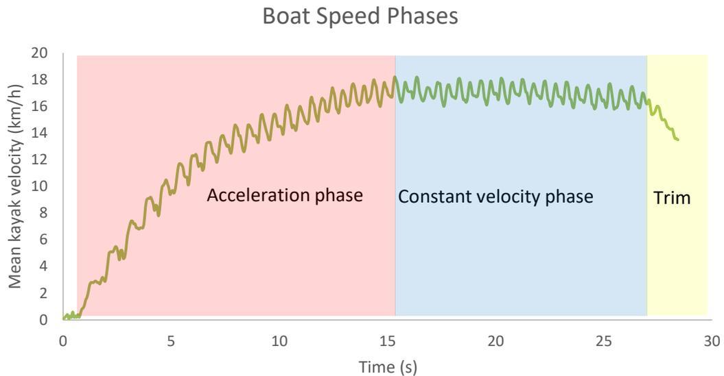
Figure 32. Boat speed phases
