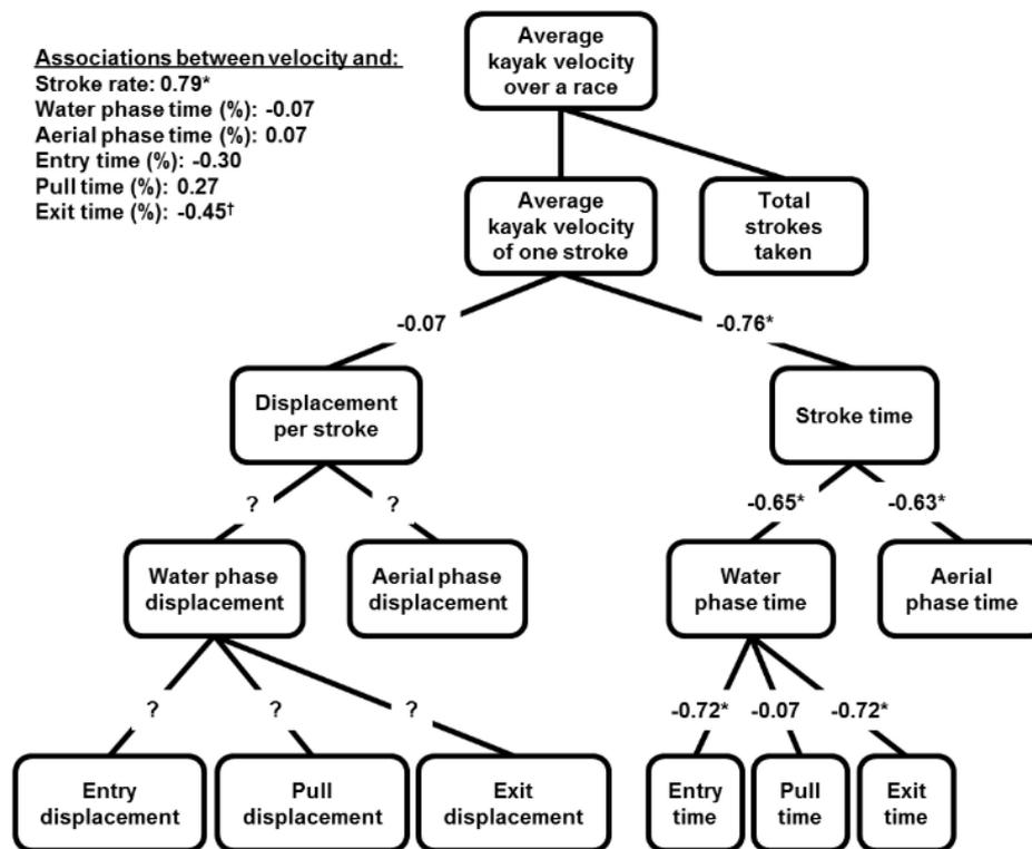
Figure 5. Kinematic determinants of kayak sprint
