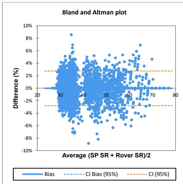
Figure 37. Bland-Altman plot of the relation between Rover GPS and SP SR
