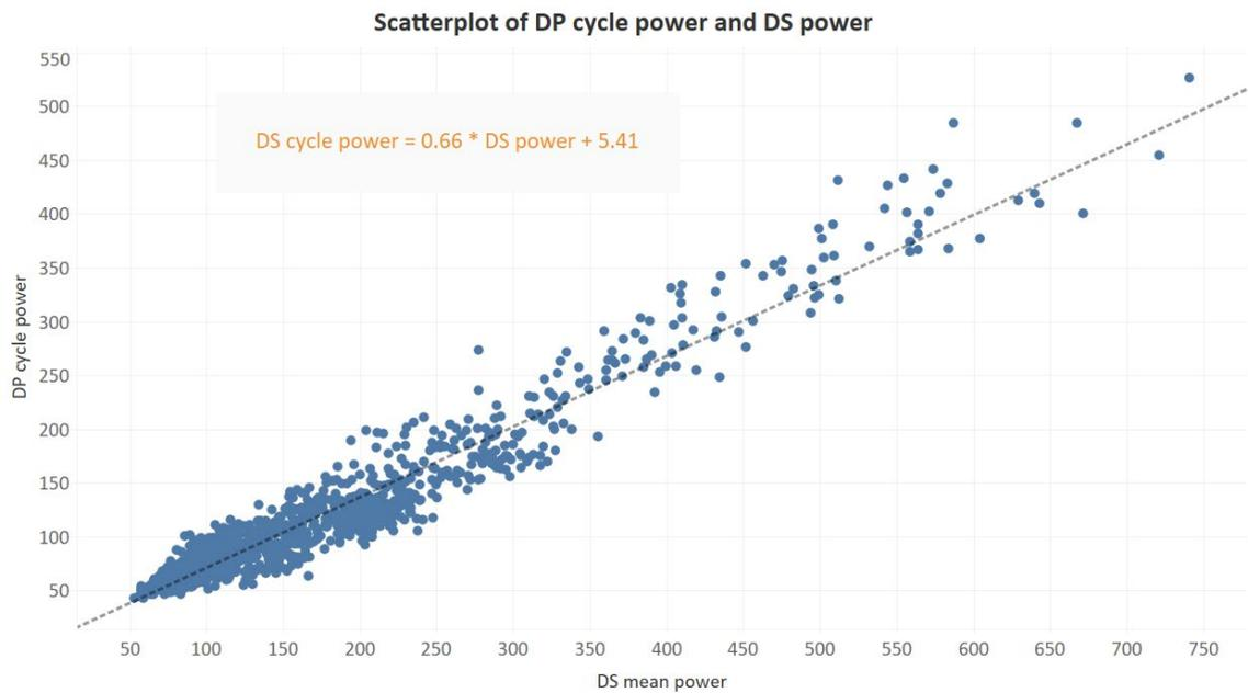
Figure 22. Regression of DP  $P_{Cycle}$  to DS  $P_{Mean}$
