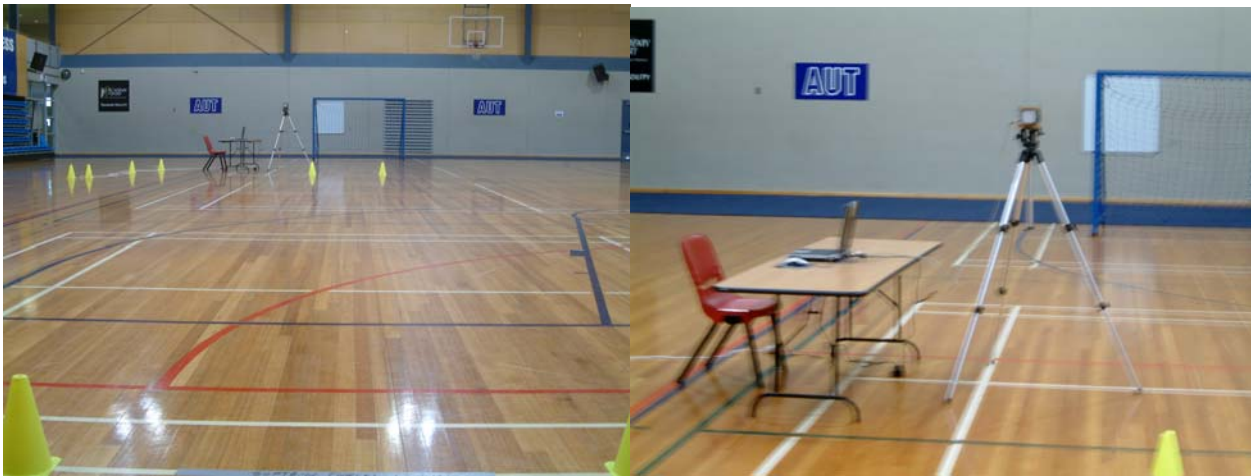
Figure 4: The positioning of the stalker radar gun, computer and marker cones indicating the throwing distance (18.4m).
