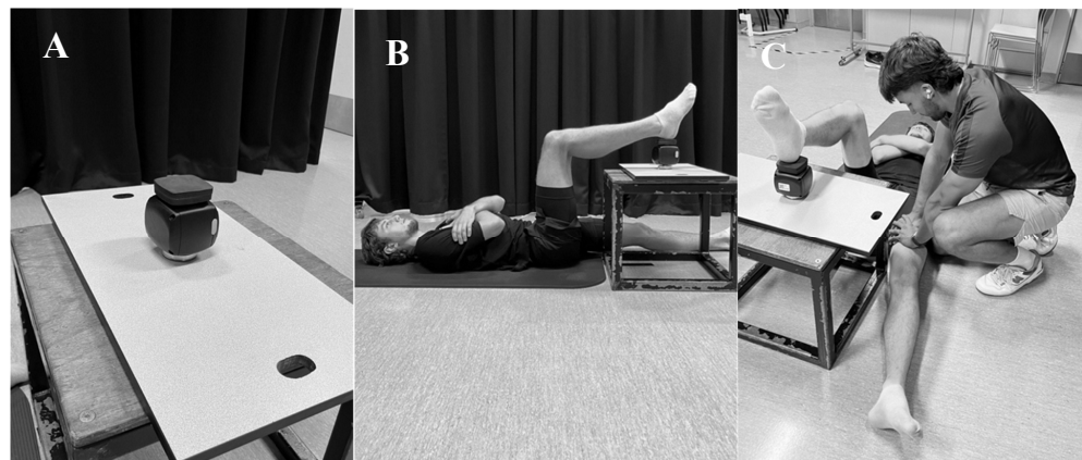
Figure 2. (A) Hawkin TruStrength attached to base plate, (B) participant set up for the 90:90 assessment, (C) tester 2 applying pressure to the non-working leg.
