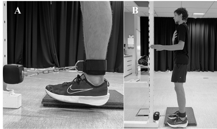
Figure 1. (A) Hawkin TruStrength attached to rack and participant's ankle. (B) Participant set up for standing hamstring assessment.
