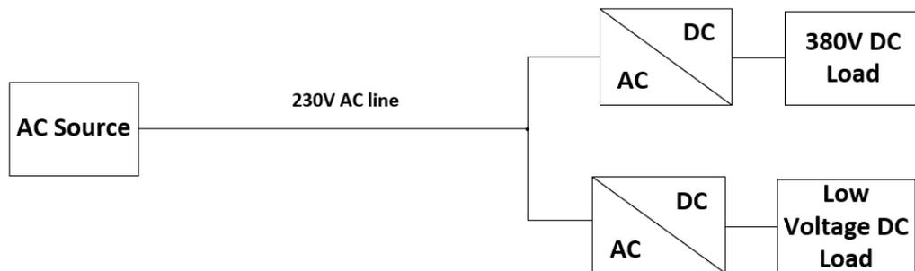
Figure 2.9: Proposed AC wiring topology 05 (Rasheed et al., 2019)
