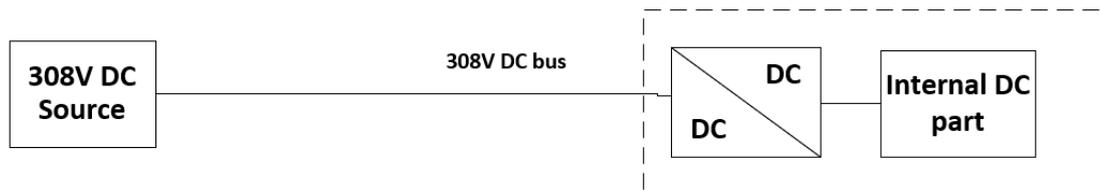
Figure 2.17: Proposed DC wiring topology 09 (Kamran et al., 2017)
