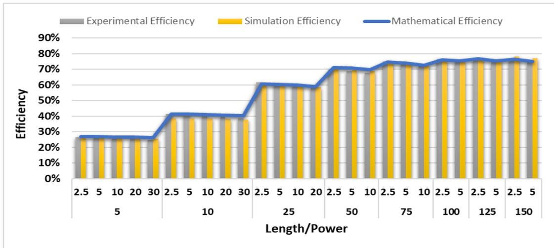
Figure 4.8: Validation charts for 24V DC wiring topology
