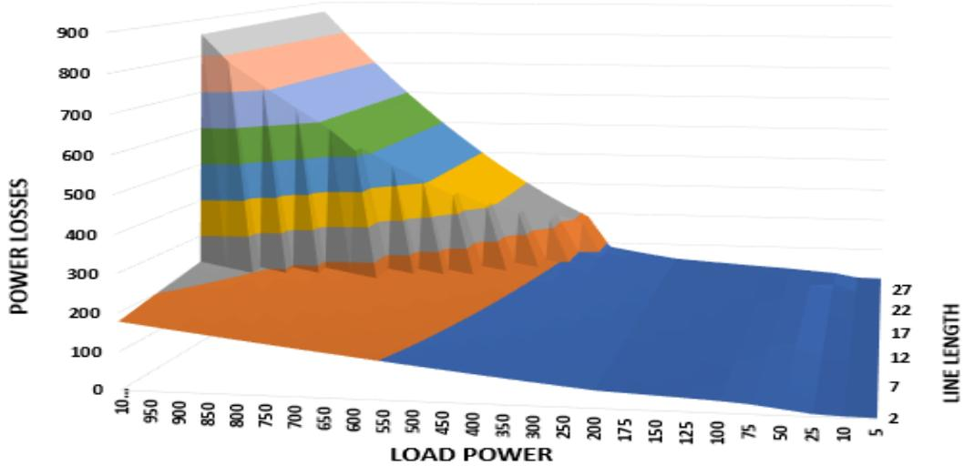
Figure 5.10: Power losses, wire length and load power chart for 4 mm<sup>2</sup>
