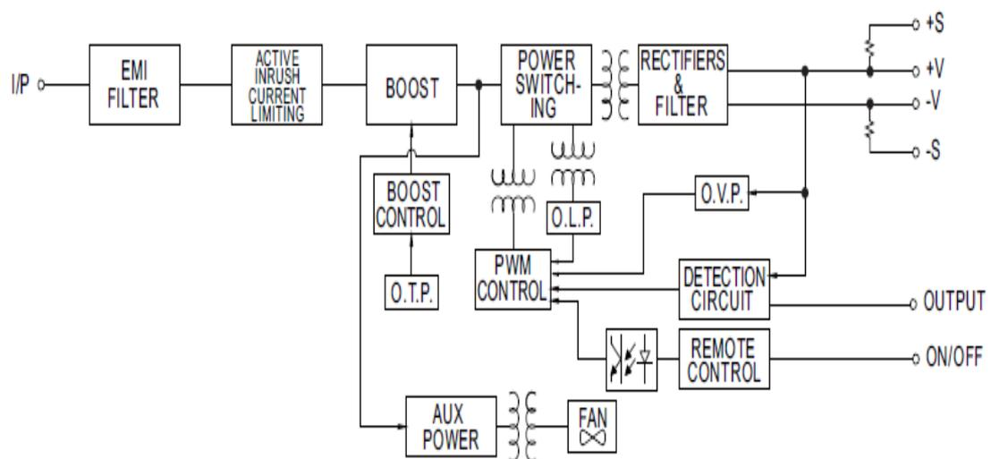
Figure 2.23: Block diagram of the DC-DC buck converter (MeanWell, 2019)
