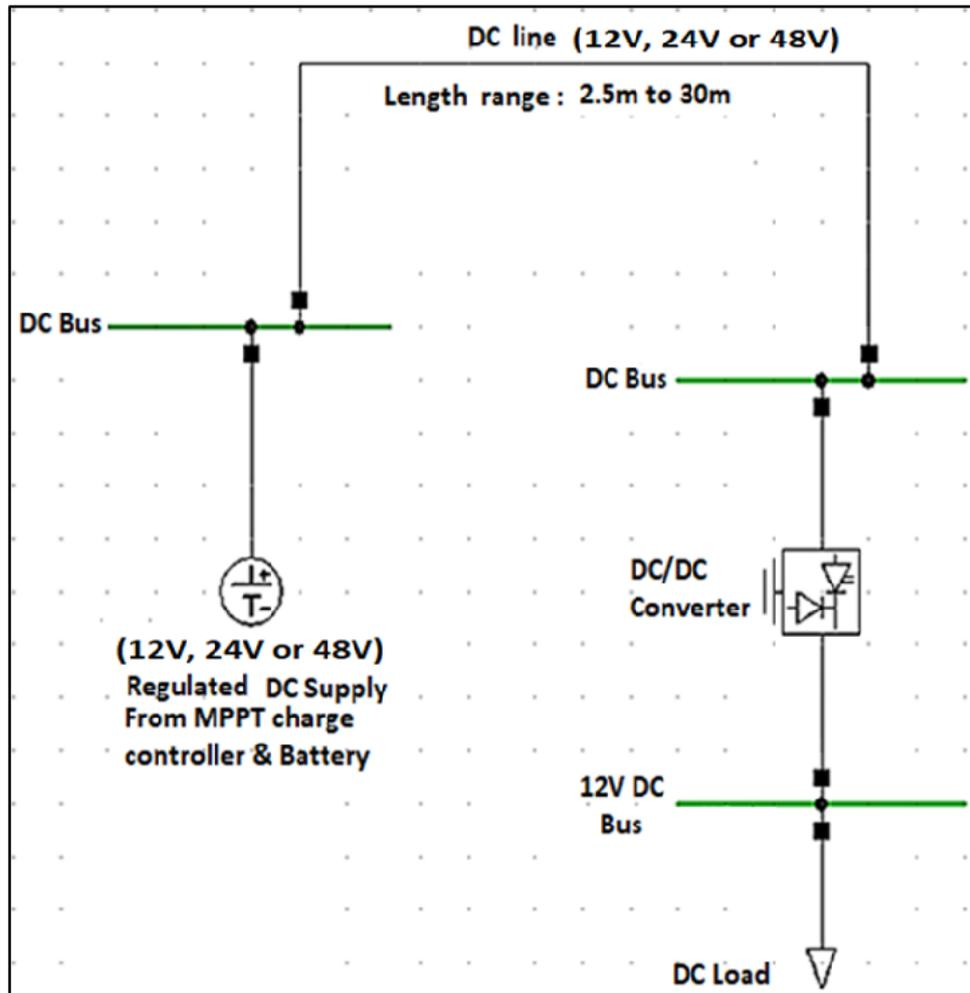
Figure 4.5: The Simulation model of proposed DC wiring topology
