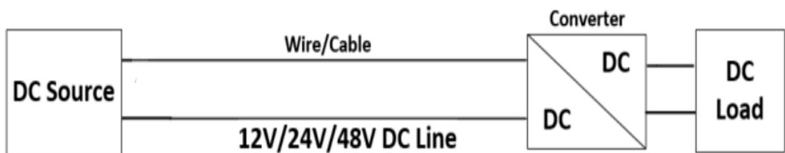
Figure 3.2: Proposed DC wiring topology in this thesis
