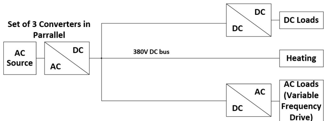
Figure 2.6: Proposed DC wiring topology 03 (Seo et al., 2011)
