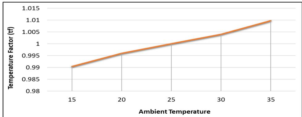
Figure 3.7 Temperature Factor ( $t_f$ ) for 12V input DC-DC Converter
