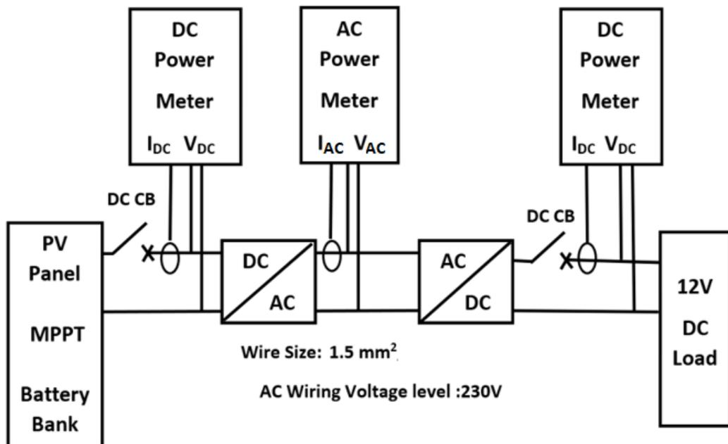
Figure 4.1: Experimental setup of proposed AC wiring topology
