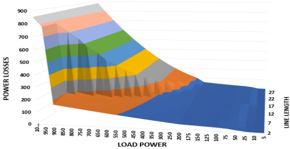
Figure 5.9: Power losses, wire length and load power chart for 2.5mm<sup>2</sup>
