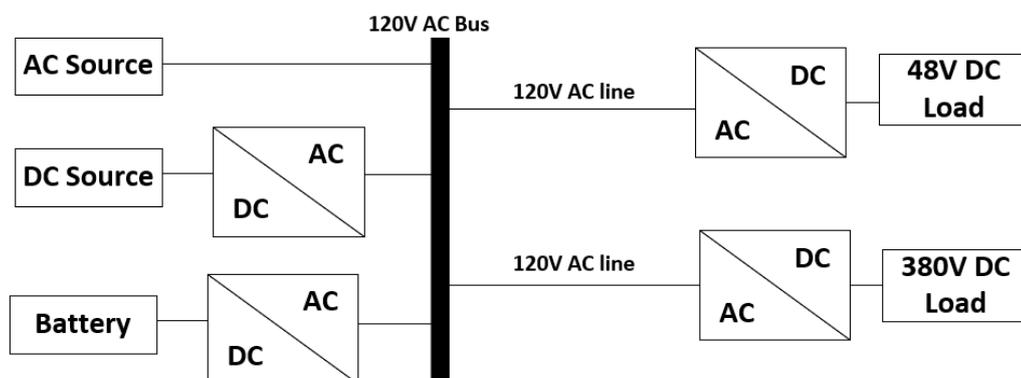
Figure 2.11: Proposed AC wiring topology 06 (Gerber et al., 2017)
