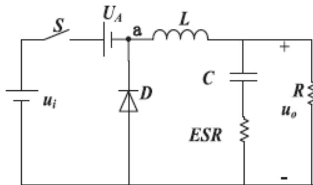
Figure 2.22: Basic DC-DC buck converter based on IGBT switches
