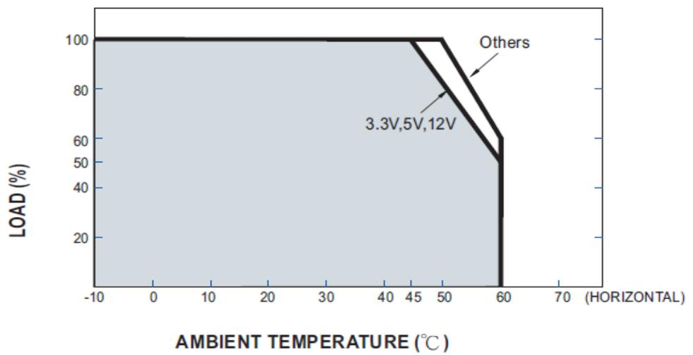
Figure 2.19 AC-DC converter de-rating curve based on ambient temperature (MeanWell, 2019)
