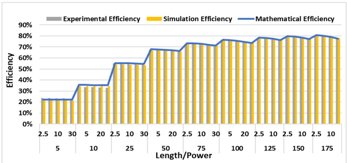
Figure 4.9: Validation charts for 48V DC wiring topology
