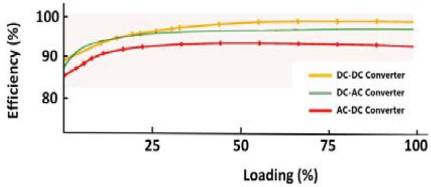
Figure 2.18: Converter Efficiency Vs % Loading (Rasheed et al., 2019)
