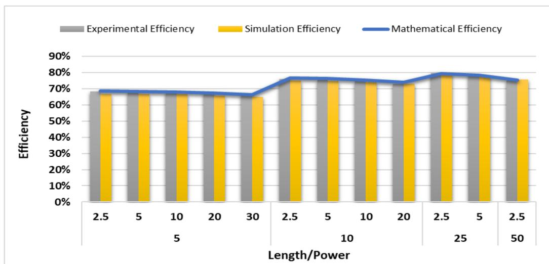
Figure 4.7: Validation charts for 12V DC wiring topology
