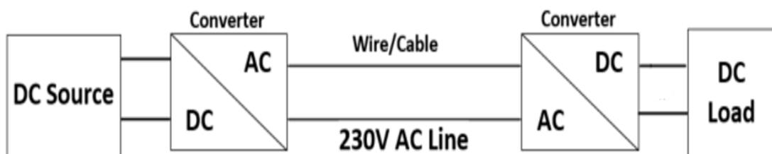
Figure 3.3: Proposed AC wiring topology in this thesis
