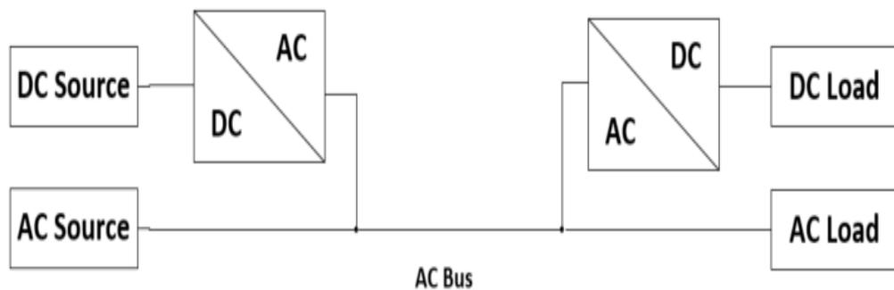
Figure 2.1: Proposed AC wiring topology 01 (D. Nilsson & A. Sannino, 2004)
