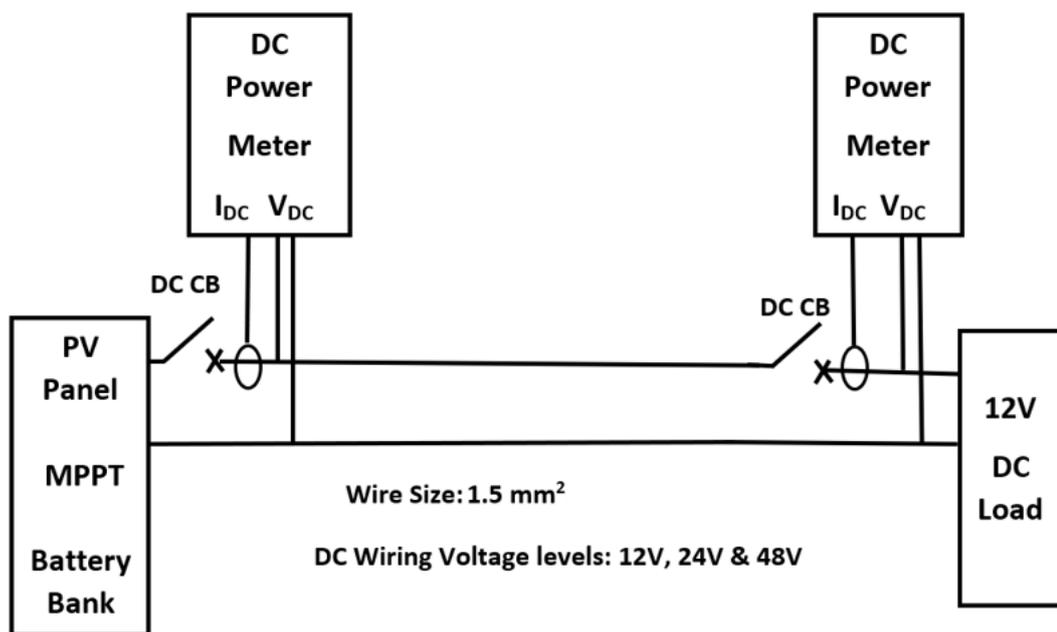
Figure 5.13: DC Wiring Topology with Standardized DC load Voltage
