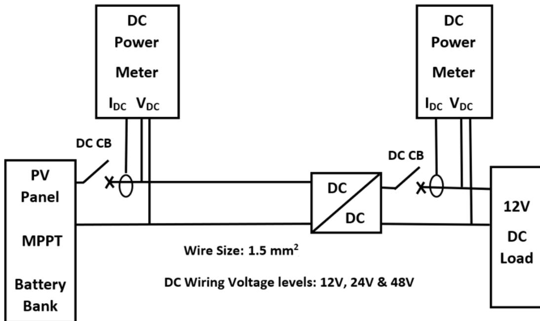
Figure 4.2: Experimental setup of proposed DC wiring topology
