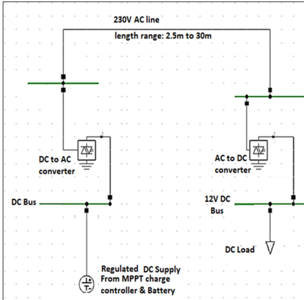
Figure 4.4: The Simulation model of proposed AC wiring topology
