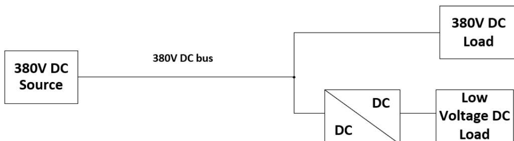
Figure 2.10: Proposed DC wiring topology 05 (Rasheed et al., 2019)
