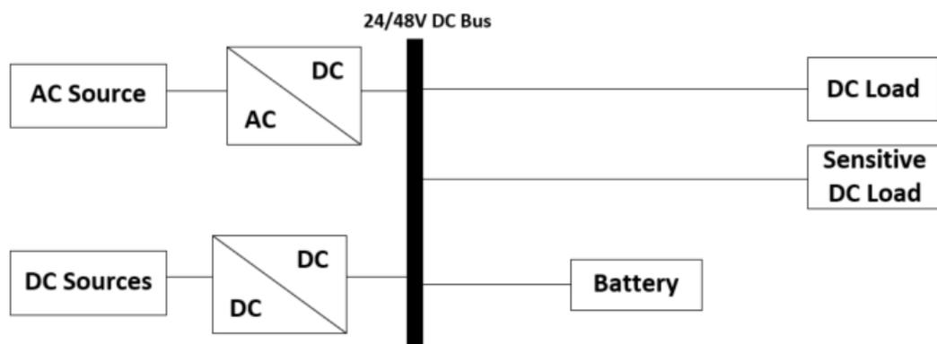
Figure 2.4: Proposed DC wiring topology 02 (Amin et al., 2011)
