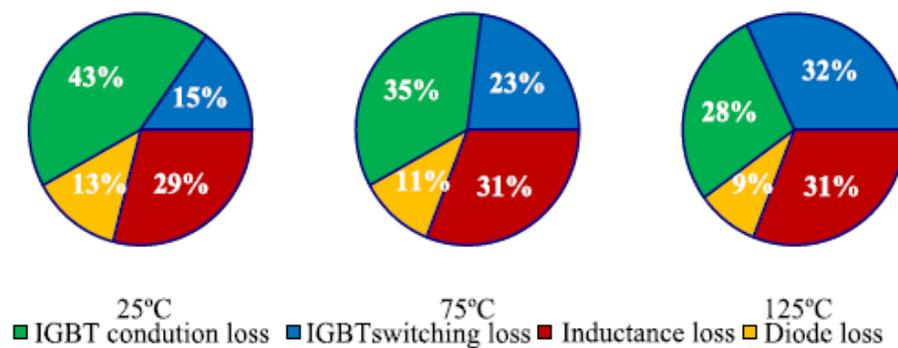
Figure 2.21: Power losses of converter components at different temperatures
