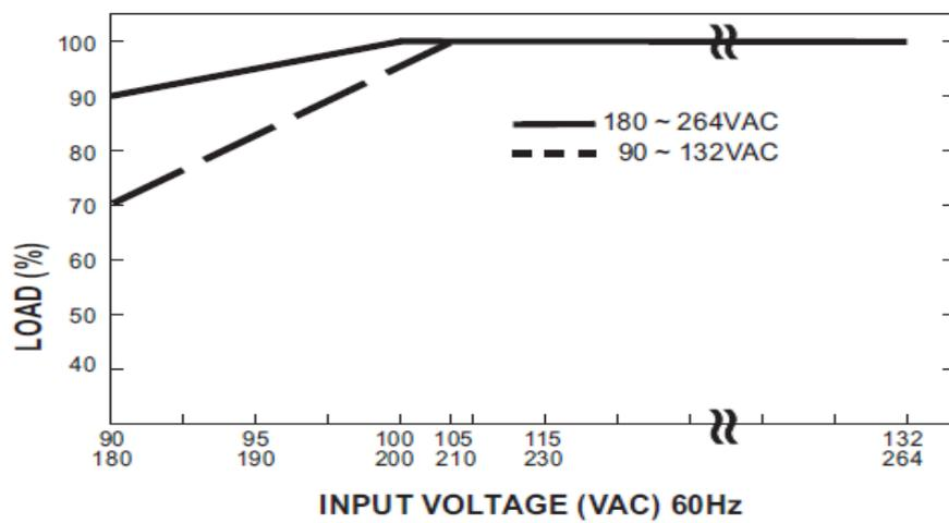
Figure 2.20 AC-DC converter de-rating curve based on input voltage (MeanWell, 2019)
