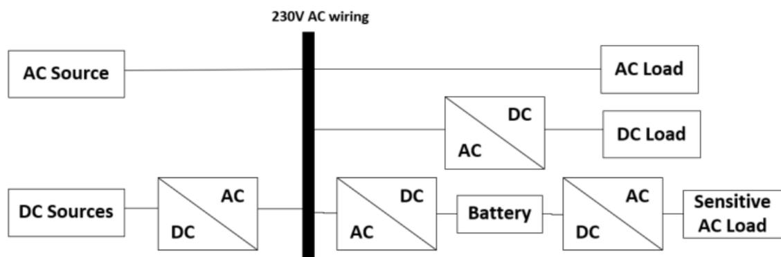
Figure 2.3: Proposed AC wiring topology 02 (Amin et al., 2011)
