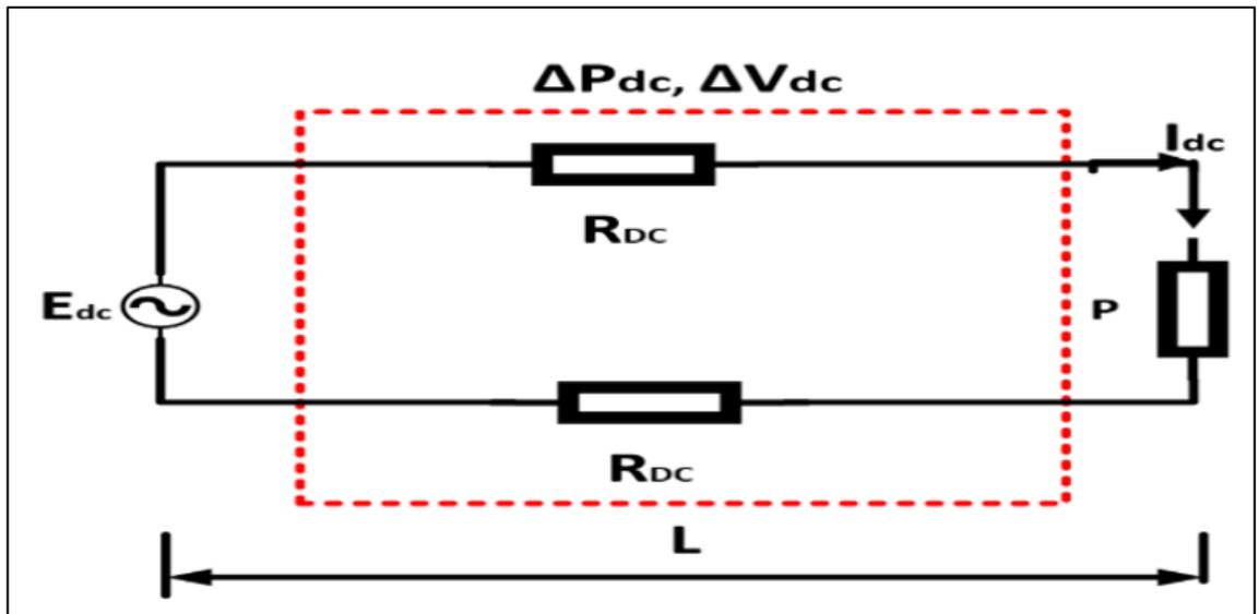
Figure 3.5: Parameters in DC power distribution system
