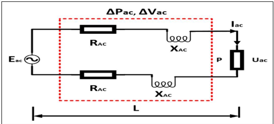
Figure 3.4: Parameters in the single-phase AC power distribution system
