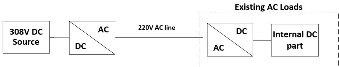
Figure 2.16: Proposed AC wiring topology 07 (Kamran et al., 2017)
