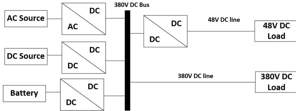
Figure 2.12: Proposed DC wiring topology 06 (Gerber et al., 2017)
