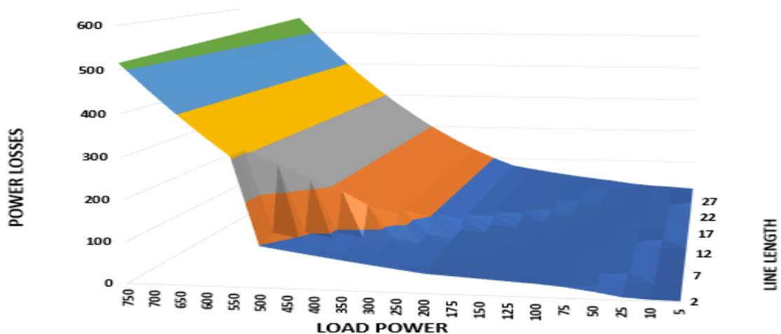
Figure 5.7: Power losses, wire length and load power chart for 1mm<sup>2</sup>
