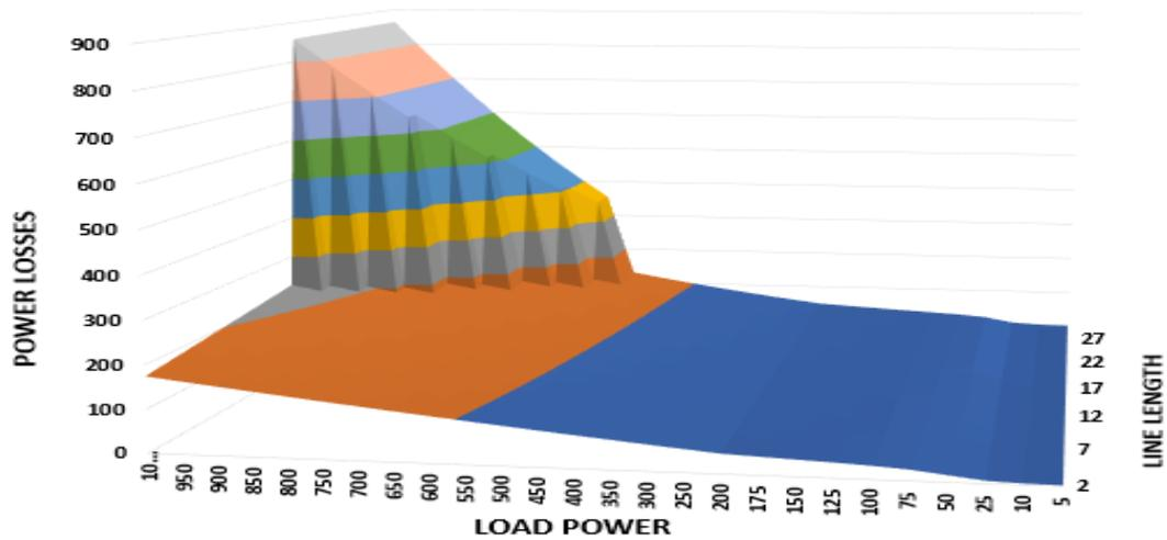
Figure 5.11: Power losses, wire length and load power chart for 6 mm<sup>2</sup>
