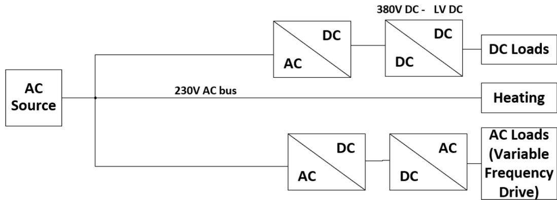
Figure 2.5: Proposed AC wiring topology 03 (Seo et al., 2011)
