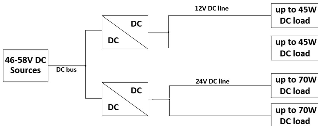
Figure 2.14: Proposed DC wiring topology 08 (Cetin et al., 2010)
