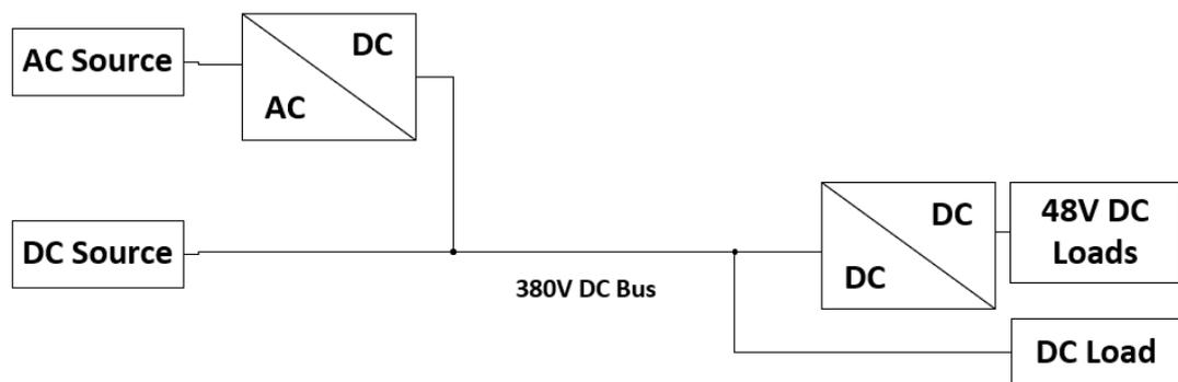
Figure 2.13: Proposed DC wiring topology 07 (Cvetkovic et al., 2012)
