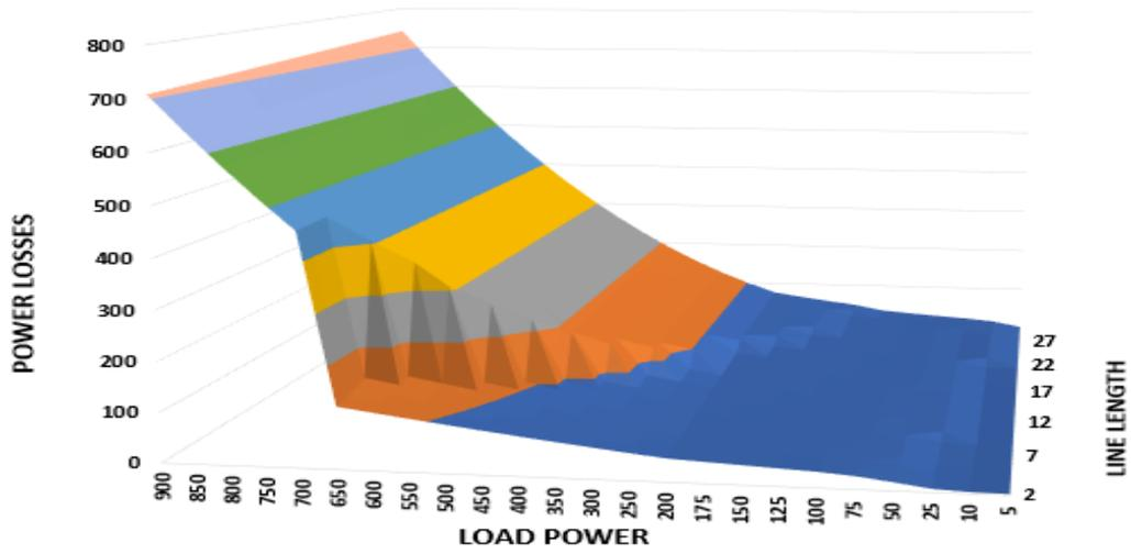
Figure 5.8: Power losses, wire length and load power chart for 1.5 mm<sup>2</sup>
