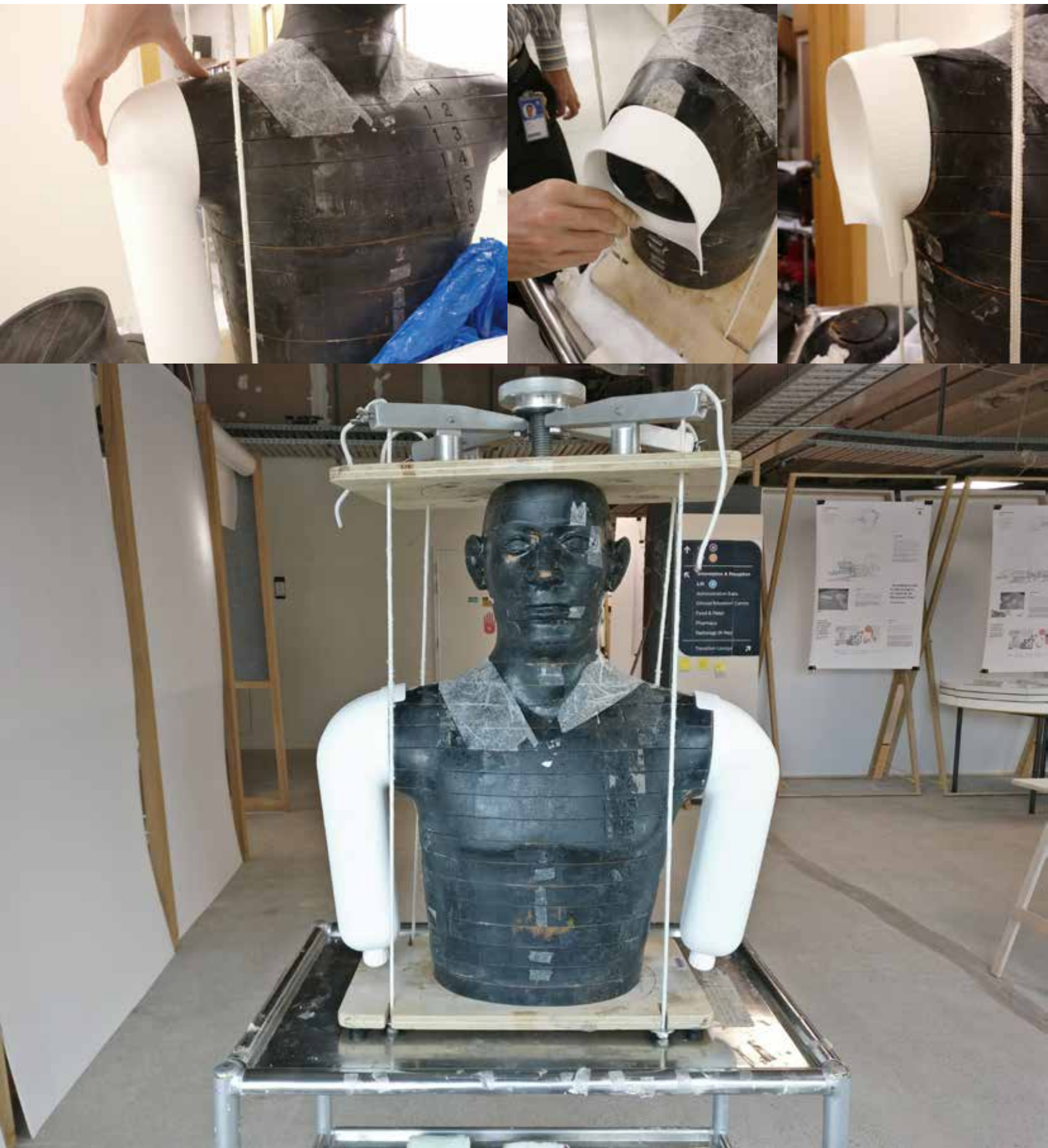
A photo showing the final 3D-printed arms being testing on the simulation model to make sure they fit correctly.
