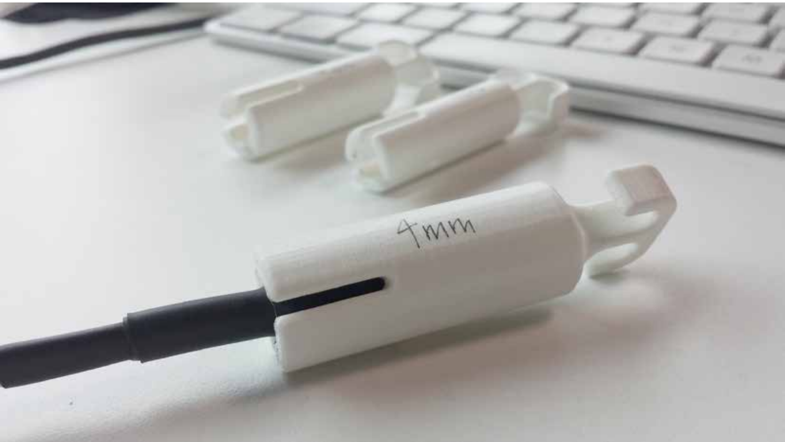
A close-up of the insulator caps design showing how the cap fits over the end of the thermometer.
