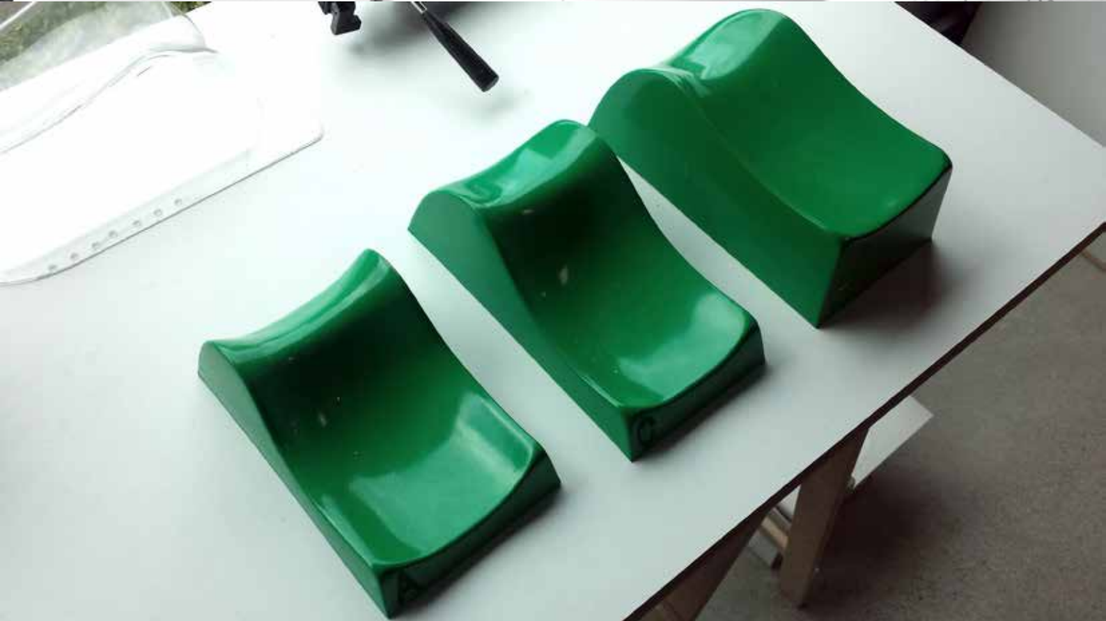
Head and neck cradle vacuum form moulds for various patient head sizes.
