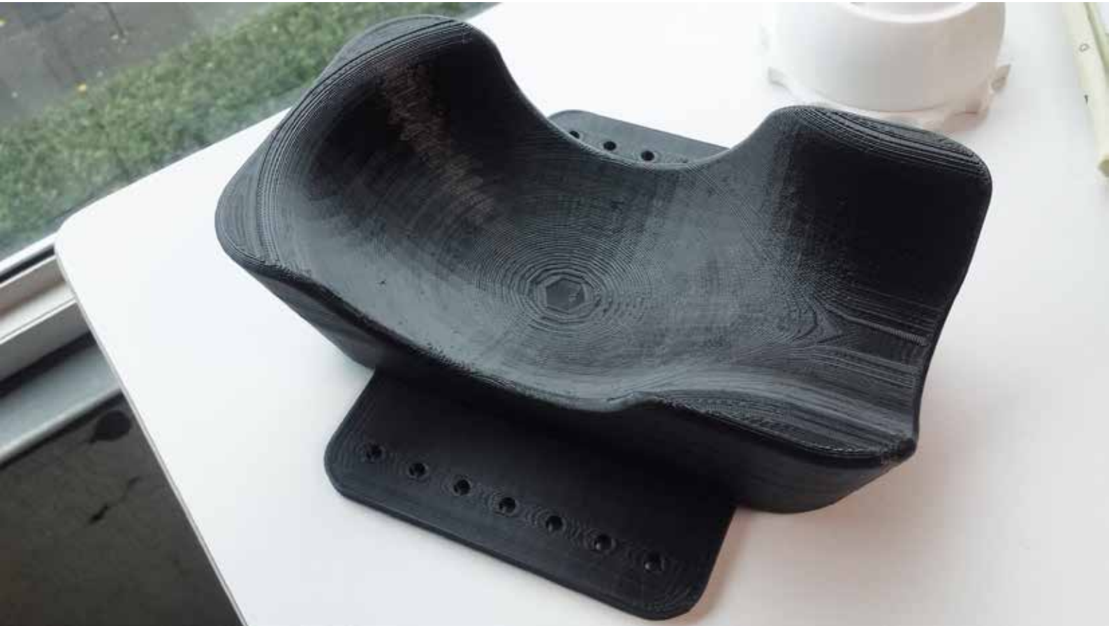
3D-printed head and neck cradle prototype used for testing and validation.
