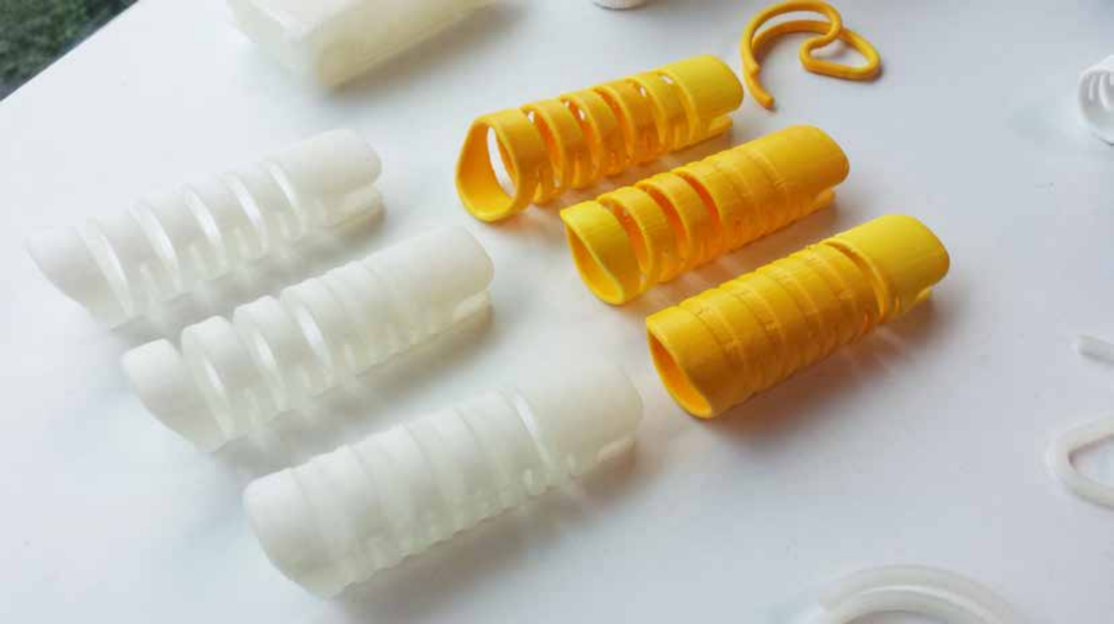
3D splints demonstrating different concentrated areas of isolation and rubber coating versus raw printed material.
