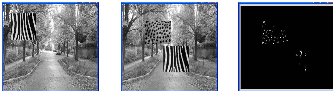
Figure 3.4 a test example of filter approach segmentation. The first image is the background image, the second image is the background image with foreground texture. The third image is the difference of the foreground image and the result image of filter approach segmentation
