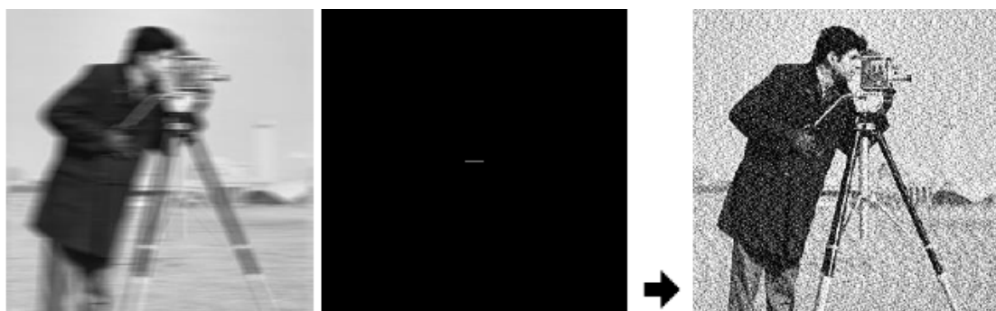
Figure 2.18 realistic refocus of horizontal motion blur cause more noise
