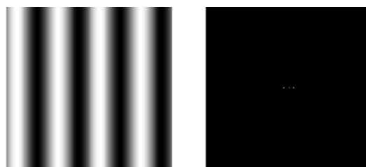
figure 2.11 a sine wave image with four sine cycles. The spectrum of this sine wave image has three pixels the distance between the center pixel and the other pixels is four pixels
