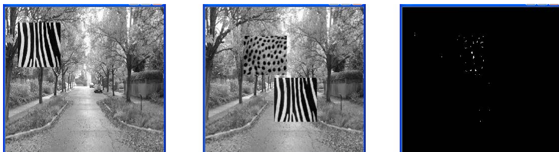
Figure 3.5 a test example of spectrum replace approach segmentation. The first image is the background image, the second image is the background image with foreground texture. The third image is the difference of the foreground image and the result image of spectrum replace approach segmentation
