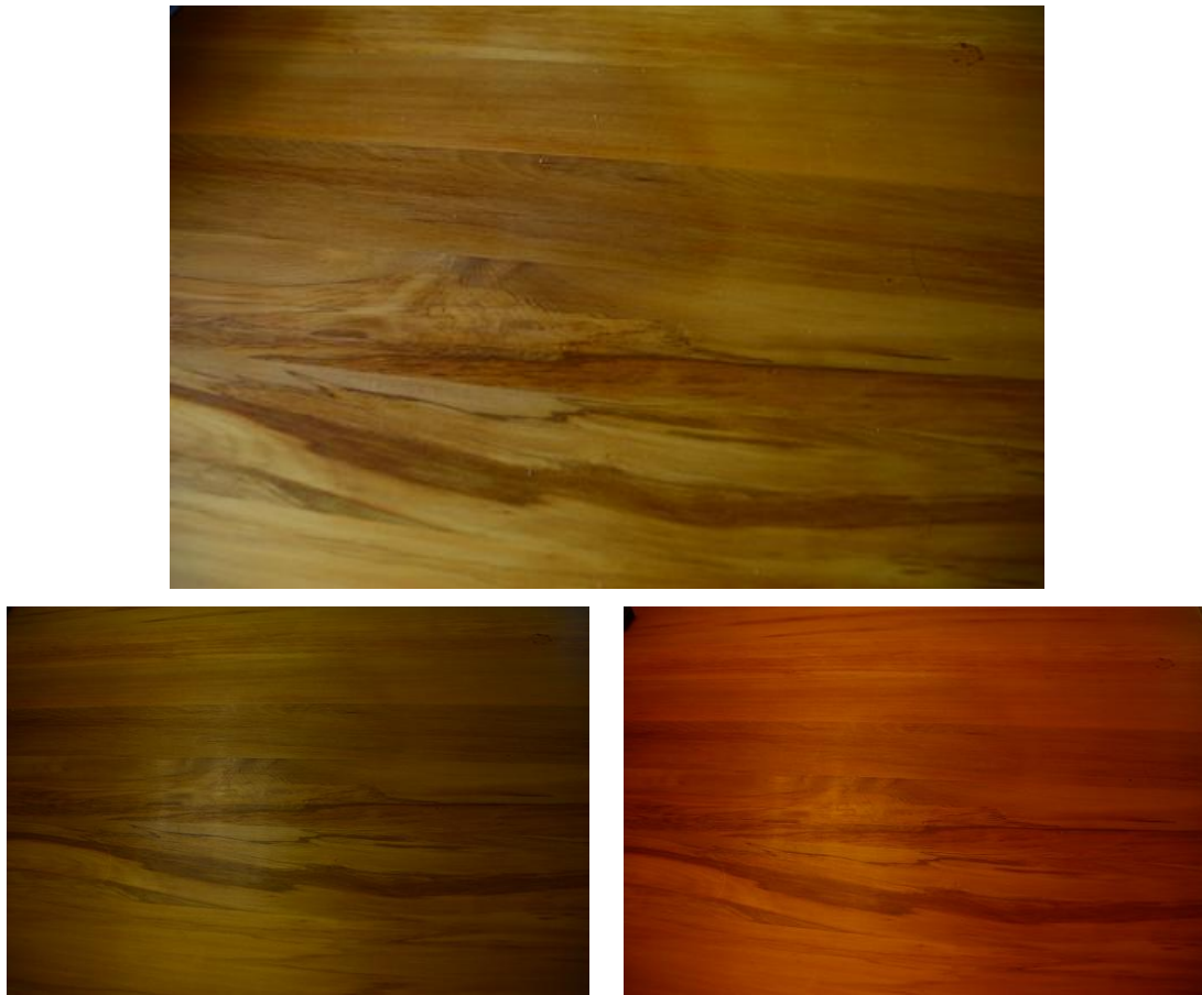
Figure 3.1 the top image was taken under the white lighting sources. The bottom two images were taken under the lighting sources with 3000k correlated colour temperature. The bottom left image was applied white balance but the bottom right image was not applied white balance.
