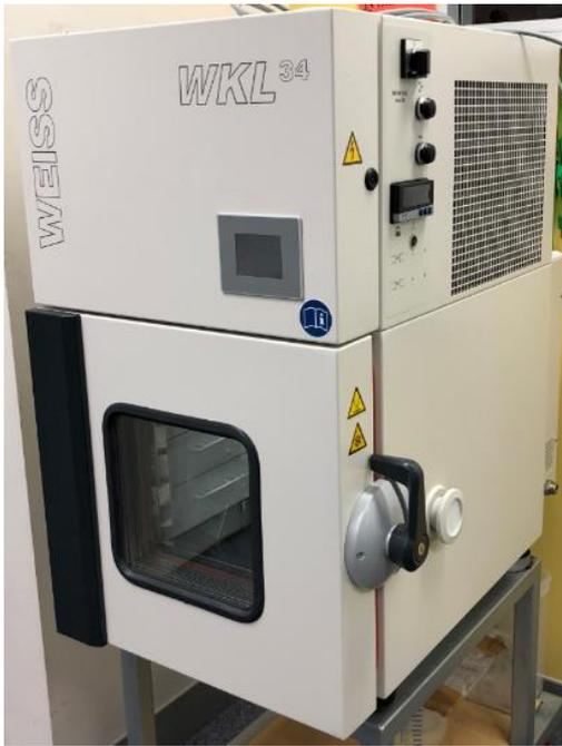
**Figure 2.19. Climate test chamber (Model: WEISS WKL34).**
