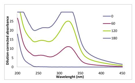
Figure 27. Wavescanning results for valine over 180 minutes reflux
