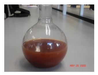
**Figure 8.** Appearance of a SMP /lactose mixture after reflux at an initial pH of 9.10 and final of 6.62.
