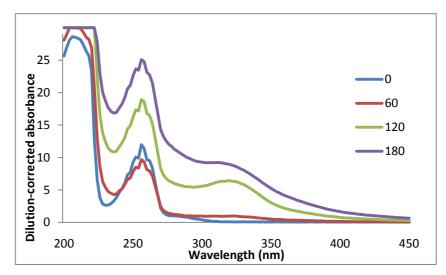
**Figure 26.** Wavescanning results for phenylalanine over 180 minutes reflux
