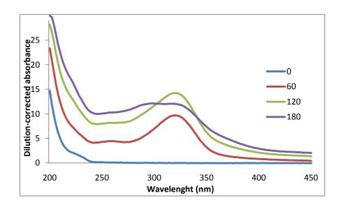
Figure 24. Wavescanning results for alanine over 180 minutes reflux
