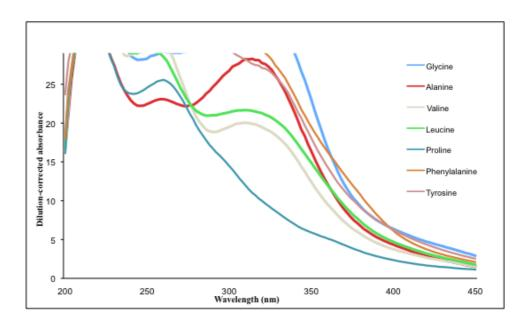
**Figure 21.** Wavescanning results for neutral non polar amino acid products after adjusting ethanol concentration to 50%
