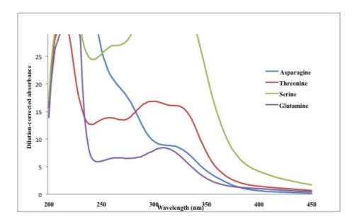
**Figure 18.** Wavelength scanning results for neutral polar amino acid products after adjusting ethanol concentration to 50%.
