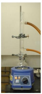
Figure 7. The standard reflux configuration with a 100 mL round bottom flask.
