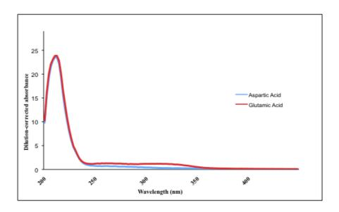
**Figure 17.** Wavelength scanning results for acidic polar amino acid products after adjusting ethanol concentration to 50%
