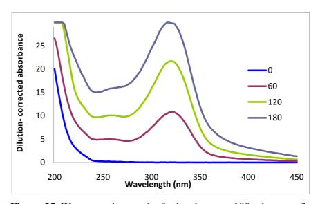
Figure 25. Wavescanning results for leucine over 180 minutes reflux
