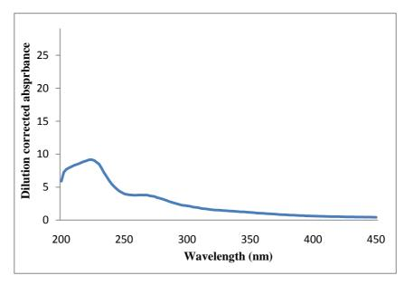
**Figure 16.** Wavelength scanning results for lactose products after adjusting ethanol concentration to 50%
