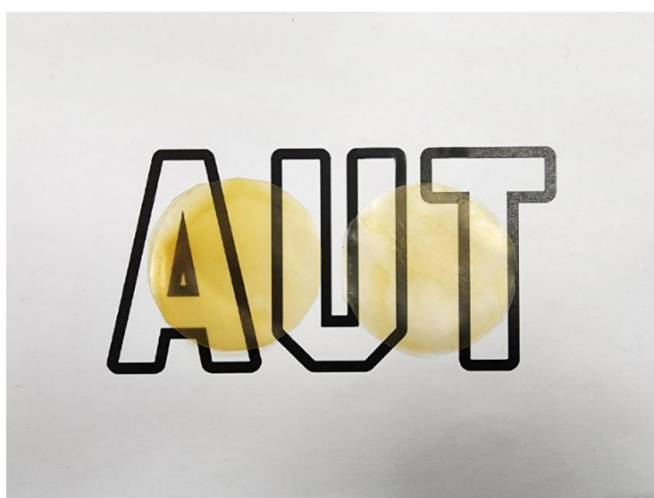
Figure 14. Oxidised WPC film (left) and normal WPC film (right).
