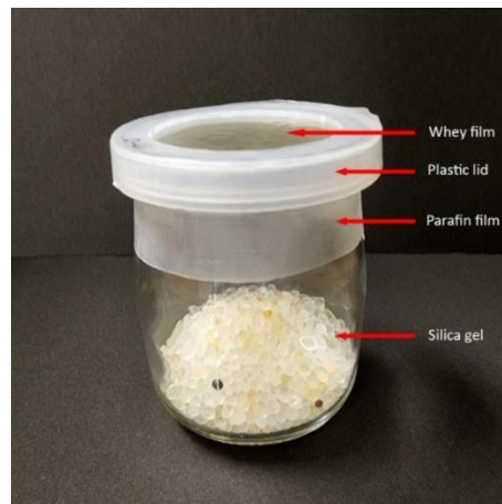
Figure 3. Set up of film sample for measuring WVP.
