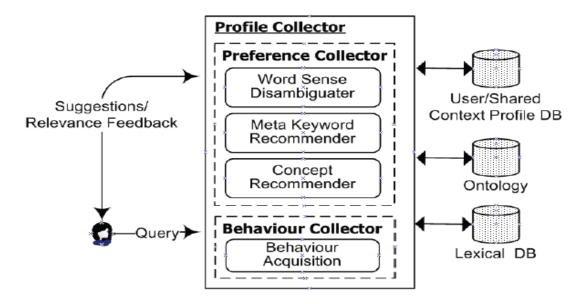
Fig. 2. Profile collector module functionality
