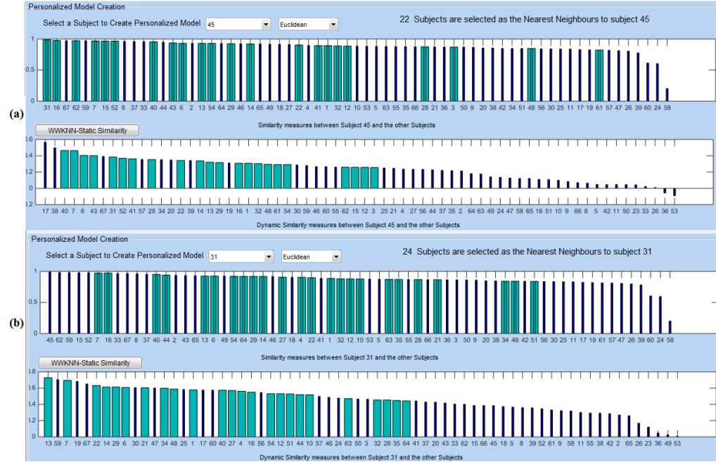
Figure 7-5 Data samples were ranked according to the integrated static-dynamic similarity to the new data from two MMT samples id: 45 and id: 31 in (a) and (b). The EEG data of the neighbour samples (shown in green) are used for training of the PSNN models.
