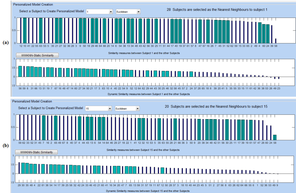
Figure 7-4 Data samples were ranked according to the integrated static-dynamic similarity to a new data from two H samples id: 1 and id: 15 in (a) and (b) respectively. The EEG data of the neighbour samples (shown in green) are used for training of the PSNN models.
