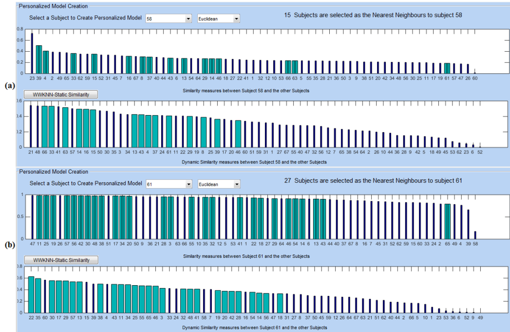
Figure 7-6 Data samples were ranked according to the integrated static-dynamic similarity to the new data from two OP samples id: 58 and id: 61 in (a) and (b). The EEG data of the neighbour samples (shown in green) are used for training of the PSNN models.
