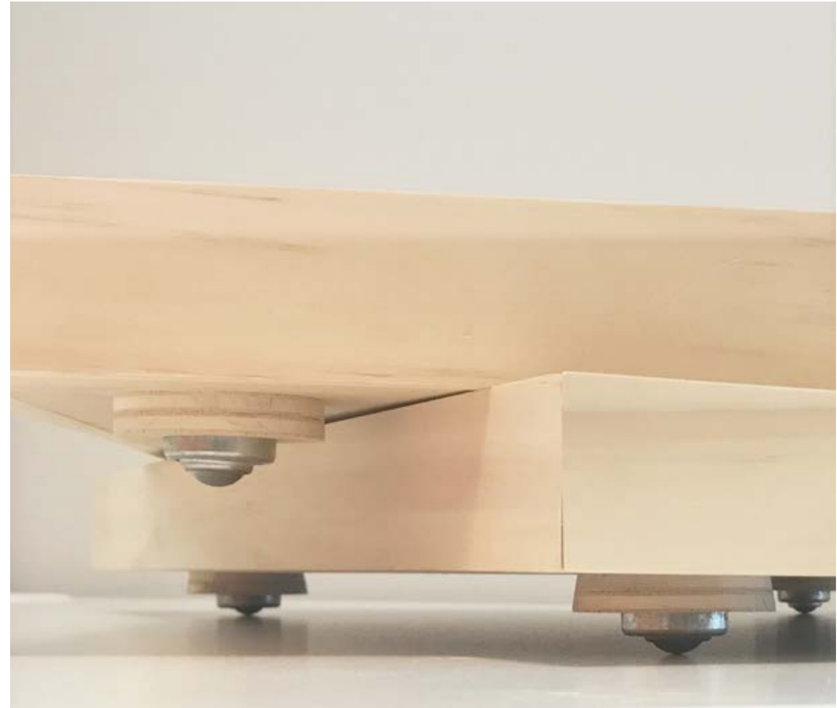
Figure 60: Ball bearings used as wheels on underside of trays.
