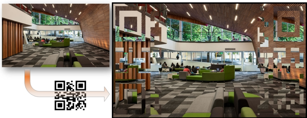
Figure 3.14: The curtain style pictorial marker design allows the QR code to be embedded on the edges of the original figure.
