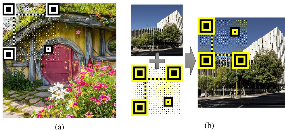
Figure 3.19: The example of transparent QR marker (a) and its encryption/decryption steps (b).
