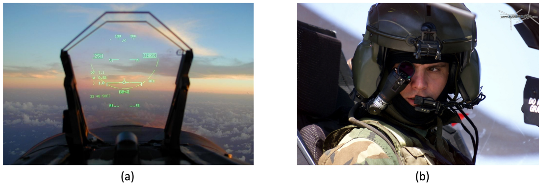
Figure 2.12: Augmented Reality is used as the military combat equipment such as in the head-up display on fighter jets (a) 1 or in integrated target engagement helmets (b) 2
