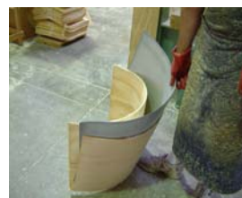
Figure 16 Investigating plywood moulding process for cushion seat backing at Libra Woodwork, Onehunga
