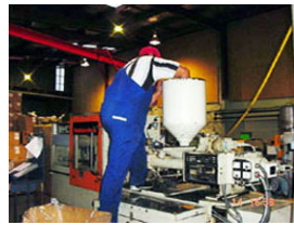
Figure 13 Investigating Injection moulding process for cosmetic cap at Plastic Solutions, Glenfield
