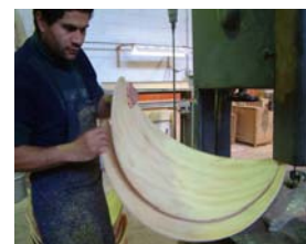
Figure 16 Investigating plywood moulding process for cushion seat backing at Libra Woodwork, Onehunga
