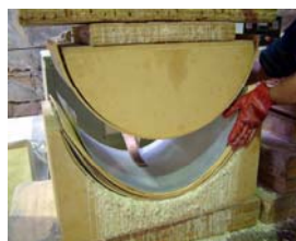
Figure 16 Investigating plywood moulding process for cushion seat backing at Libra Woodwork, Onehunga
