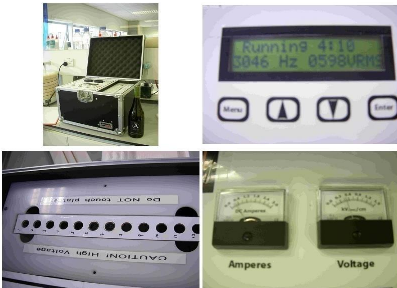
Figure 14 The static WAM. Test tubes containing the liquids under study are held in the numbered rack (lower left), and the frequency and voltage are adjusted by the digital control (top right)
