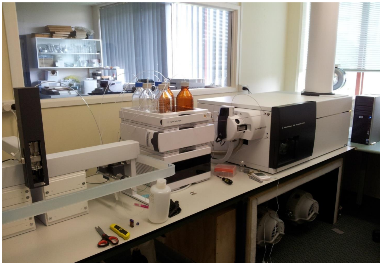
Figure 44 An Agilent 1290 Infinity UPLC - MS
