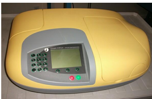
Figure 15 An GE Amersham Ultrospec 2100 Pro UV/Vis spectrophotometer
