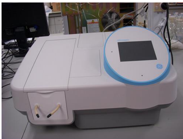
Figure 16 A GE Healthcare Ultraspec7000 UV/Visible spectrophotometer
