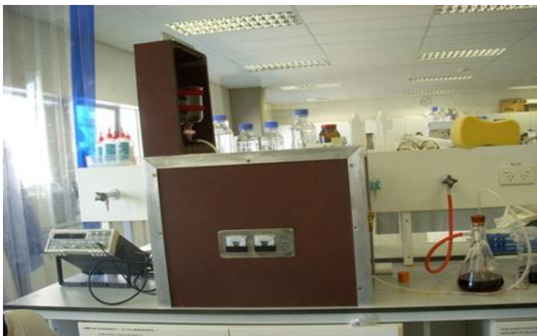
Figure 12 The flow through WAM. In this (second) configuration, the wine was pulled through the tubing by vacuum. For the first configuration the peristaltic pump (not shown) was located across the silicone tubing just visible below the reservoir
