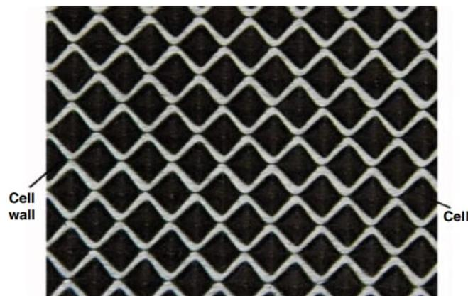
Figure 2.33: Gravure cell under microscopy [25].
