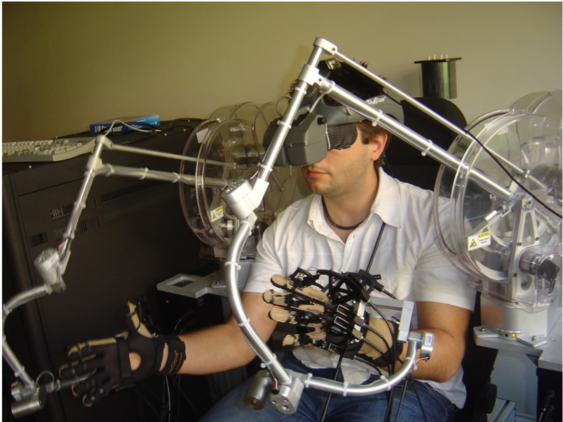
Figure 1. The Haptic Workstation by CyberGlove Systems. One example of a force reflecting haptic interface. Note the complex mechanical systems involved.
