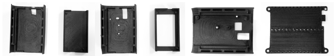
Figure 14. Developments of arm casing utilising affordable and quick 3D printing for rapid prototyping. Note the incremental addition and refinement of mounting holes and supports.
