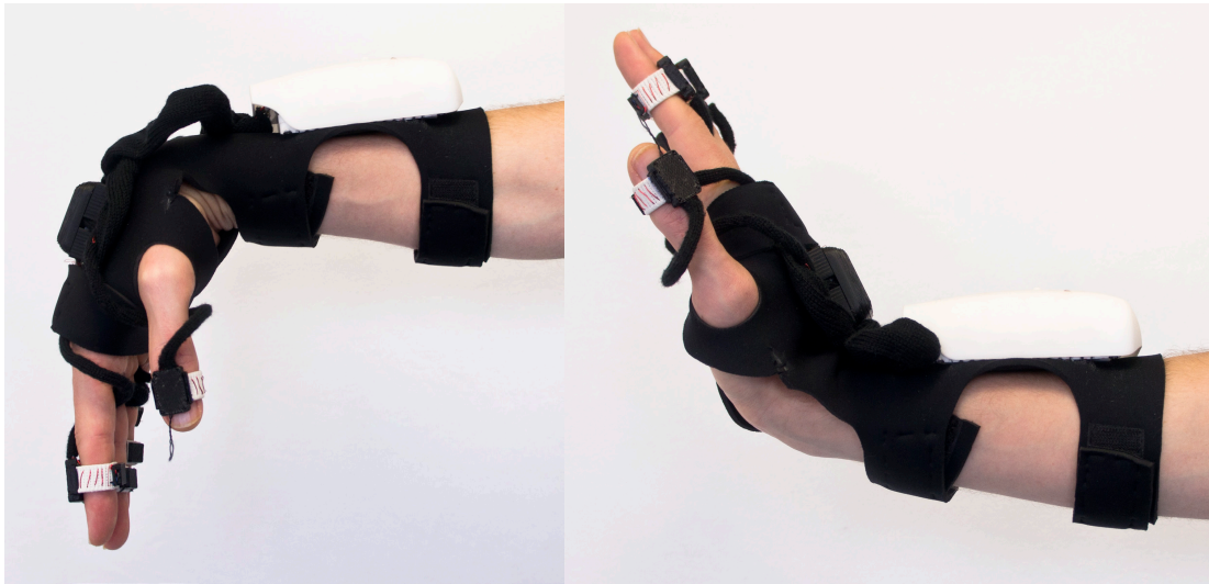
Figure 35. Testing to ensure the final prototype did not restrict range of motion of the hand and wrist.
