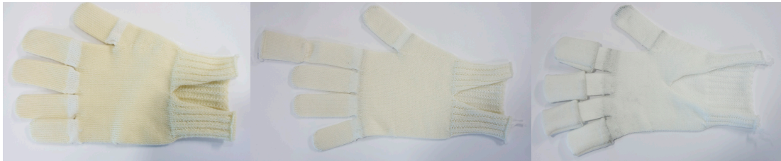
Figure 22. Glove samples with thermoplastic yarn and sleeves for electronics. The thermoplastic yarn can be seen as white strips near the join between the fingers and hand.
