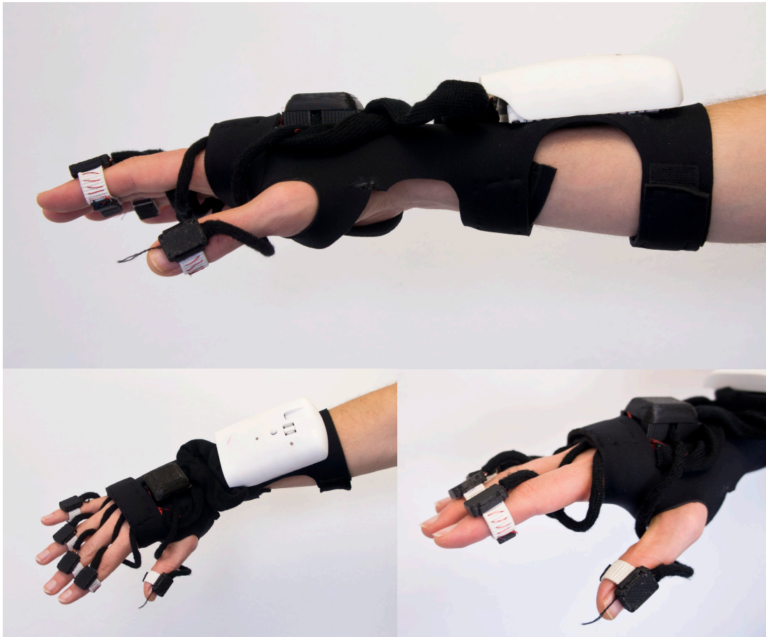
Figure 37. The final prototype. Note the positioning of sensor and motor modules on the middle phalanges of the fingers and the distal phalange of the thumb.
