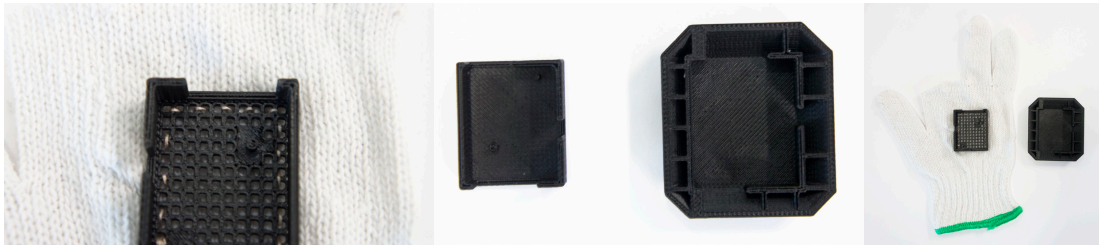
Figure 19. Early iterations of wrist casing. Note the use of a grid pattern in the base to allow for stitching to the textile component.
