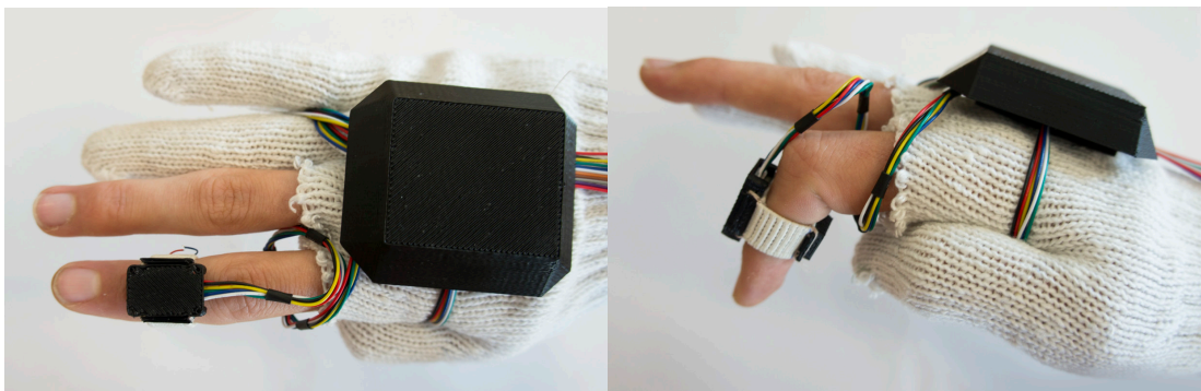
Figure 27. Early development of solid wire connections. Note how the wire is looped around the finger to provide a structure to guide it back to the original shape when compressed.
