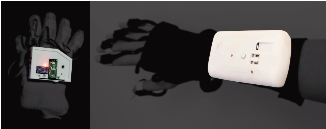
Figure 7. Repositioning of primary module. The highlighted module on the back of the hand (left) was redesigned to become the highlighted arm module (right).
