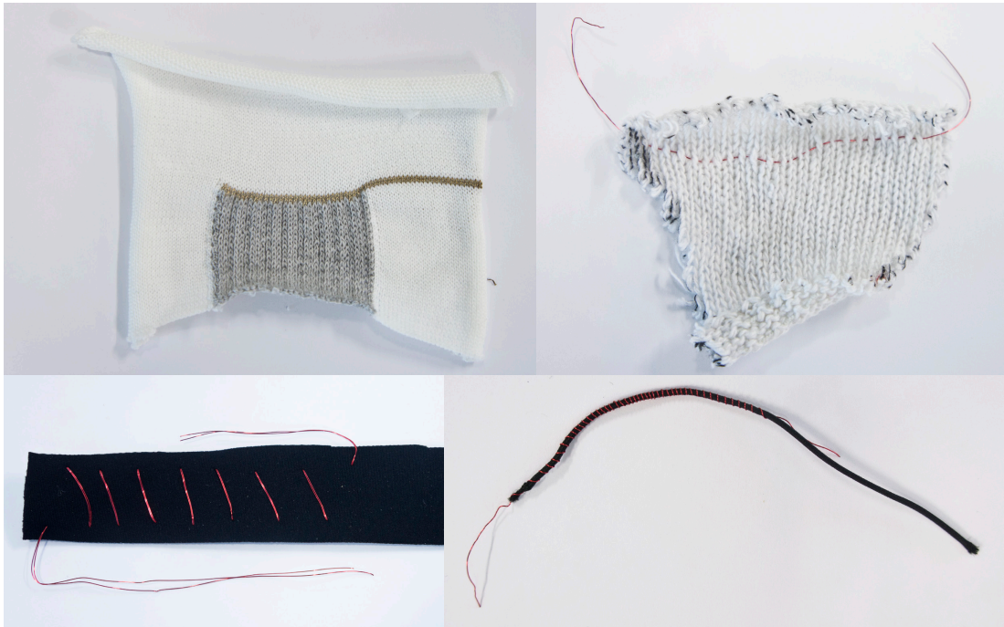
Figure 28. Early investigations into flexible wiring. Clockwise from top left: conductive yarn, enamelled wire threaded into a knitted textile, enamelled wire coiled around an elastic core, and stitched as a coil into neoprene.
