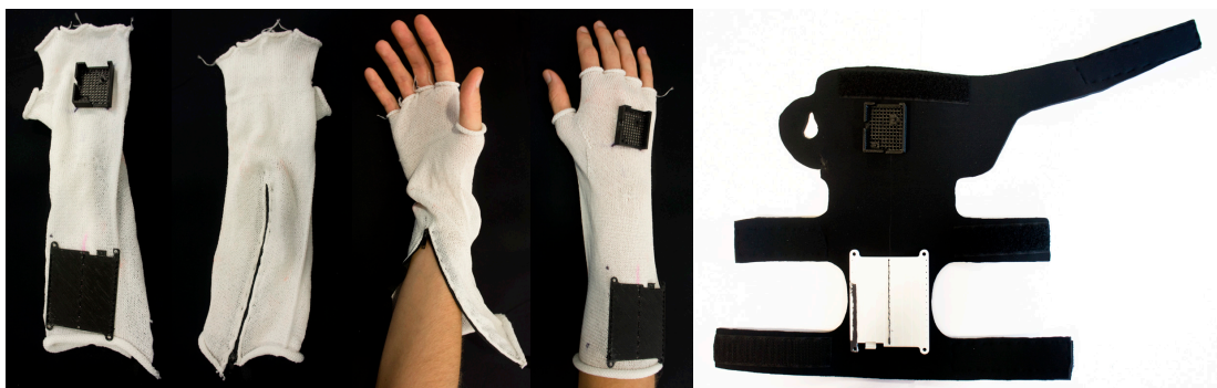
Figure 26. Final versions of the knitted glove with zipper and neoprene wrap.
