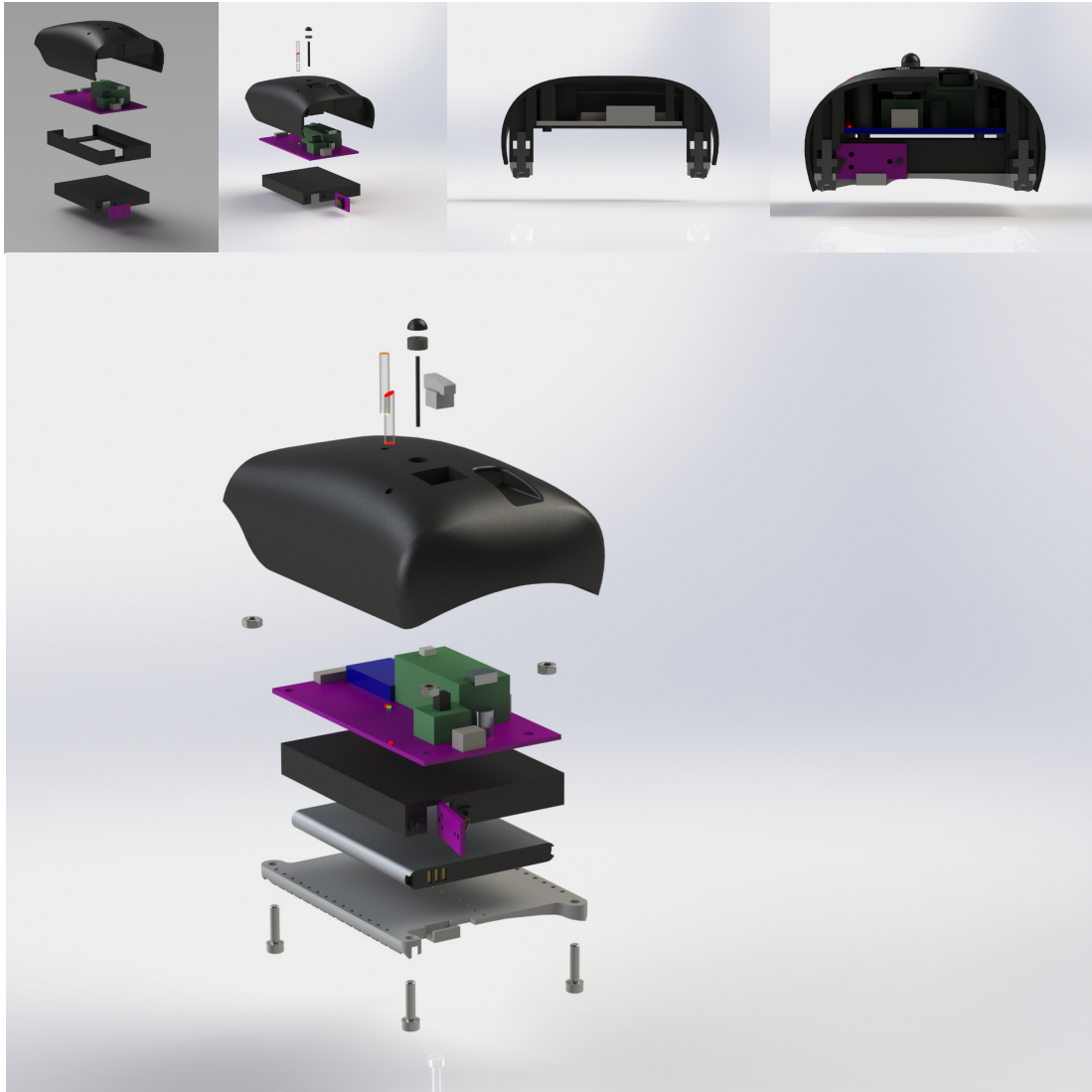
Figure 15. CAD images at different stages of development. Exploded views and cutaways were utilised to check for interference between different parts of the assembly.
