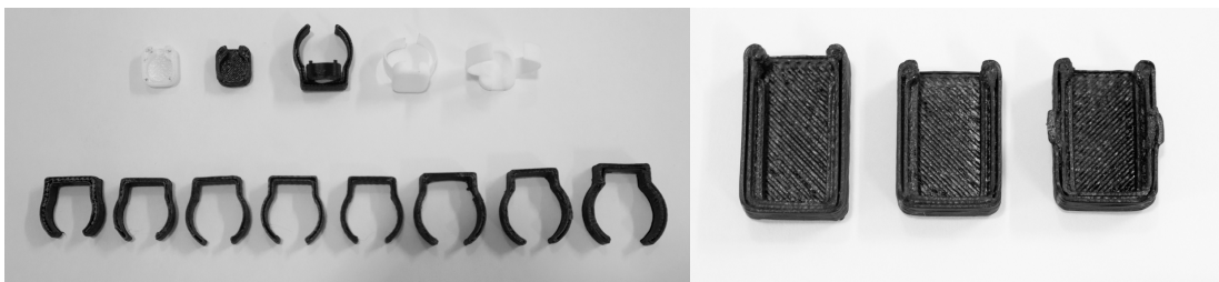
Figure 8. Iterative refinement of plastic sensor housing and haptic motor clips. In order to obtain a comfortable but firm fit, different clip sizes were made to suit a range of finger sizes.
