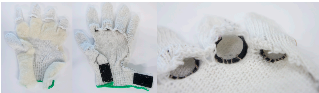
Figure 21. Initial glove developments. Early developments explored ways of opening up the palm area of the glove and supporting the finger entry points with plastic rings.
