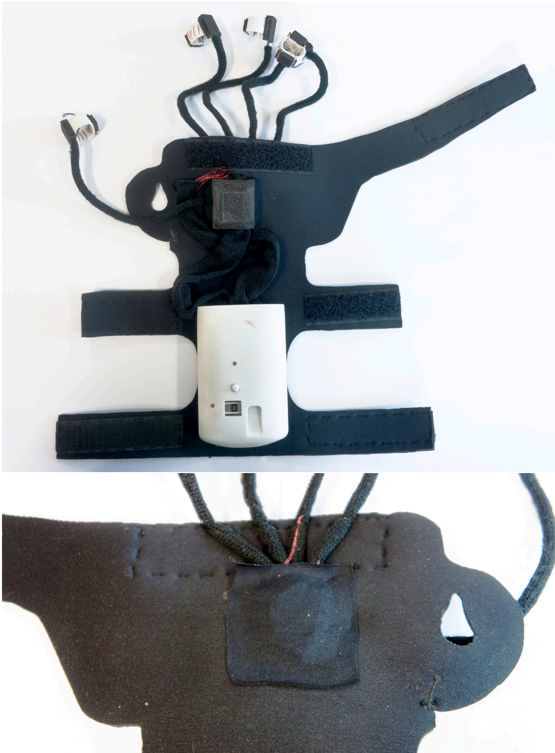
Figure 36. Final tweak. A patch was glued over excess enamelled wire. The wire bundles from the finger modules can be seen stitched in place at the top of the neoprene in the bottom image.
