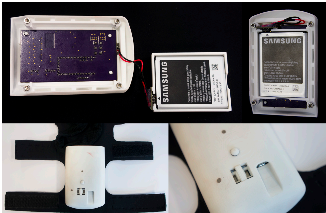
Figure 17. Final arm module assembly. The battery can be seen mounted on the underside before the module is attached to the neoprene support.
