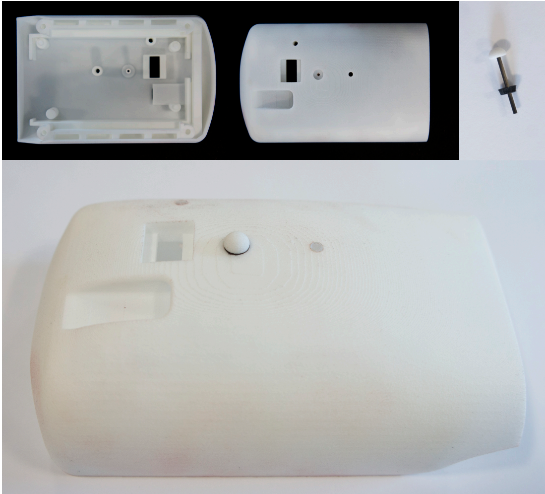
Figure 16. High quality 3D printed arm casing and push button actuator assembly. A piece of carbon fibre rod and a small piece of foam was attached to a 3D printed dome to form the push button actuator assembly (centre image). Note the fine details produced with this rapid prototyping method.
