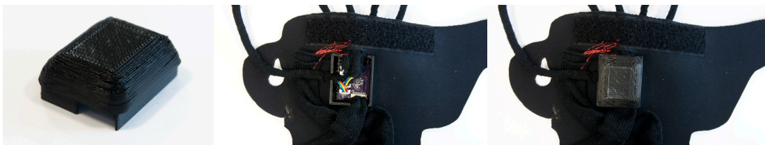
Figure 20. Final assembly with redesigned top cover. Note the reduced size of the cover.
