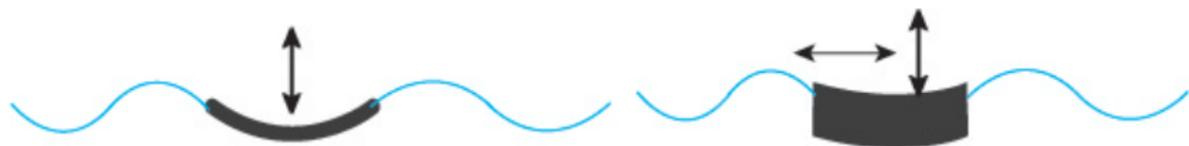
*Need the velocity potential along the draft: vertical distance between the waterline and the bottom of the plate.*
