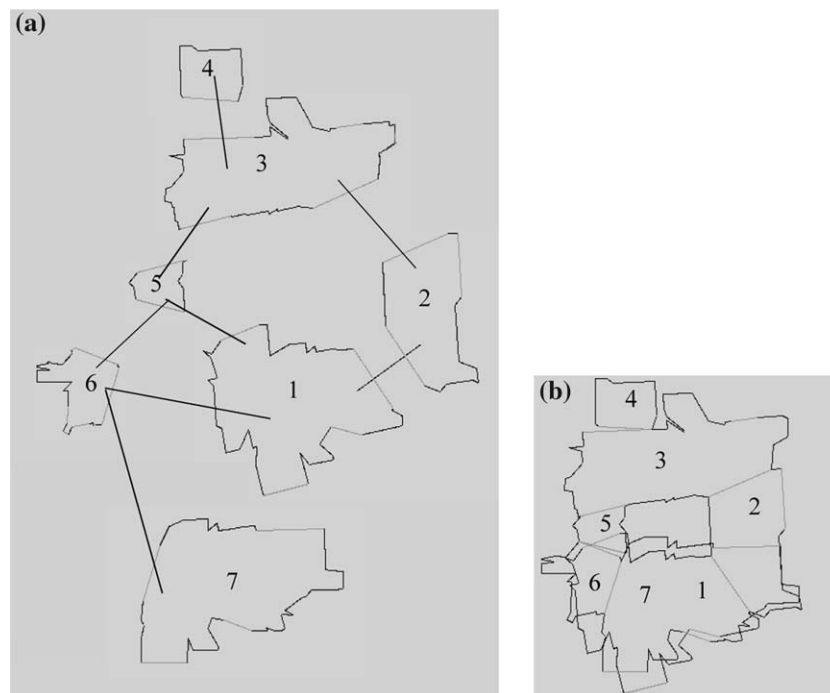
Fig. 6. (a) and (b) The topological and global maps, respectively. The robot is in ASR7. ASR7 clearly covers most of ASR1 in (b). It passes the centre crosscheck and a match is thus indicated.
