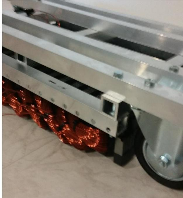
Figure 7.1 Close-up of Chassis Design using Castors
