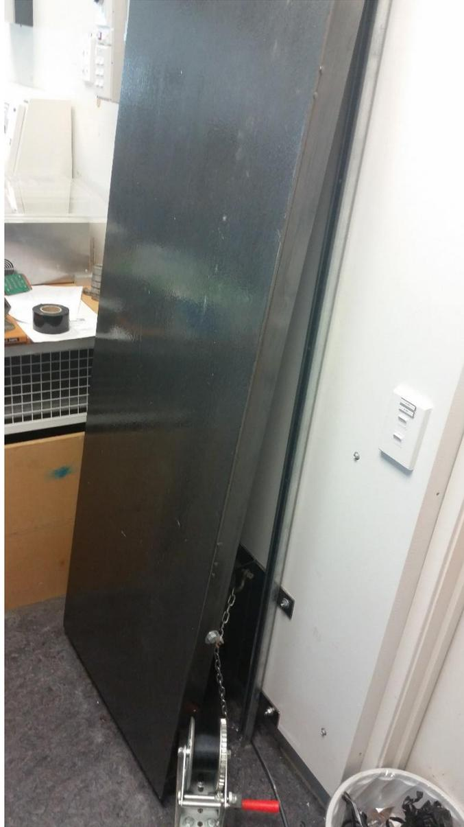
Figure 6.8 Maximally Erect Steel Backing Plate (86°)
