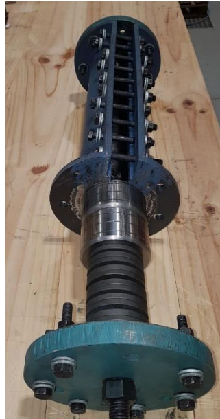
Figure 5. 3. Self-centring Structural Connector (SSC).
