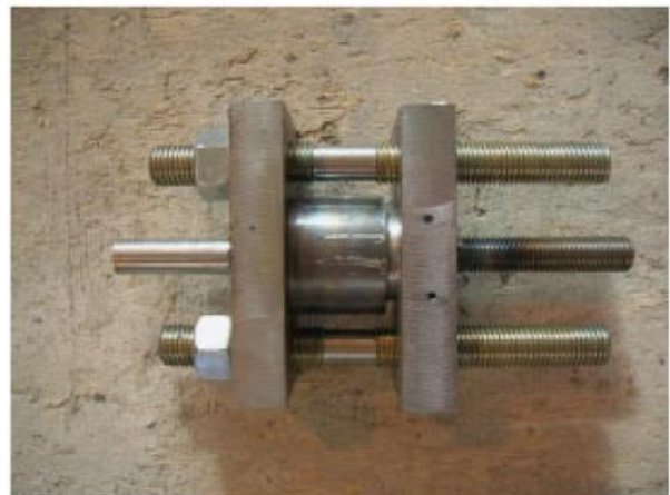
Figure 1. 18. High Force to Volume (HF2V) dampers [16, 47]
