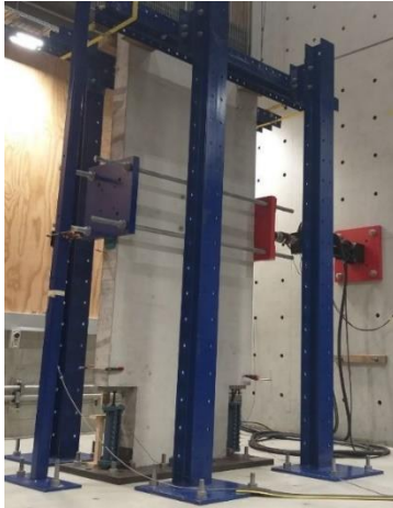
Figure 4. 13. Experimental Verification: (a) RSFJ shear wall, and (b) SSC shear wall.
