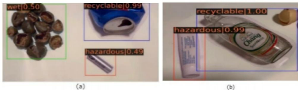
Figure 7.7 Transformer-based classification results from videos (a) the results of classifying battery, can, and chestnut, which also belong to hazardous waste, recyclable waste, and wet waste respectively (b) the classification results of glass bottle and ointment, which also belong to hazardous waste and recyclable waste
