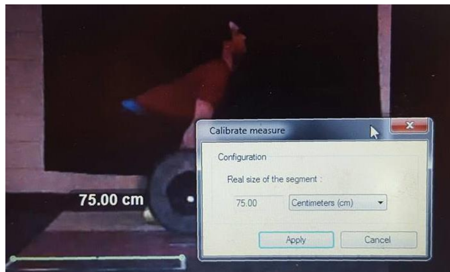
Figure 9 Calibration of measuring stick
