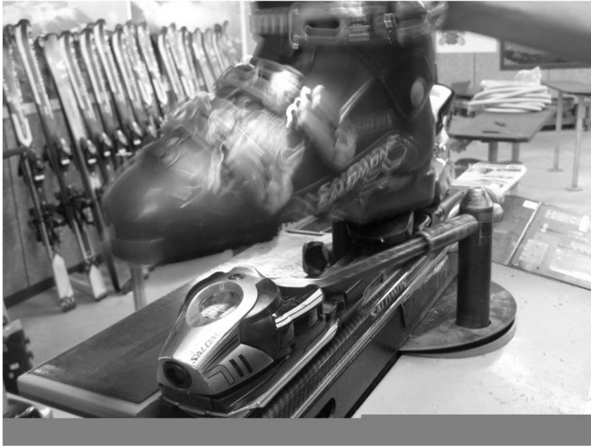
Figure 5.6: Wintersteiger machine torque testing the toe-piece in Mz twist.
