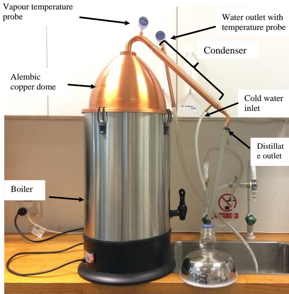
**Figure 9.** An Alembic copper pot still for distillation of rum.
