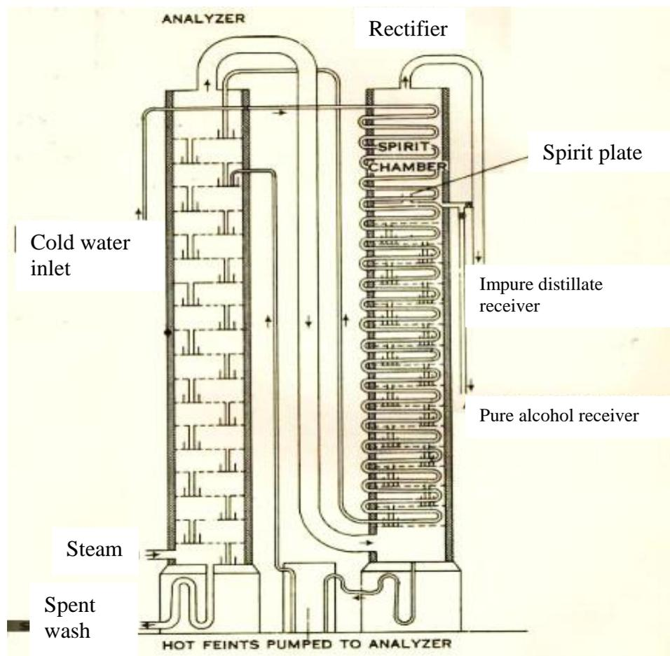
**Figure 6.** Column Still for production of Rum (The Whisky Exchange - AA, 2013).
