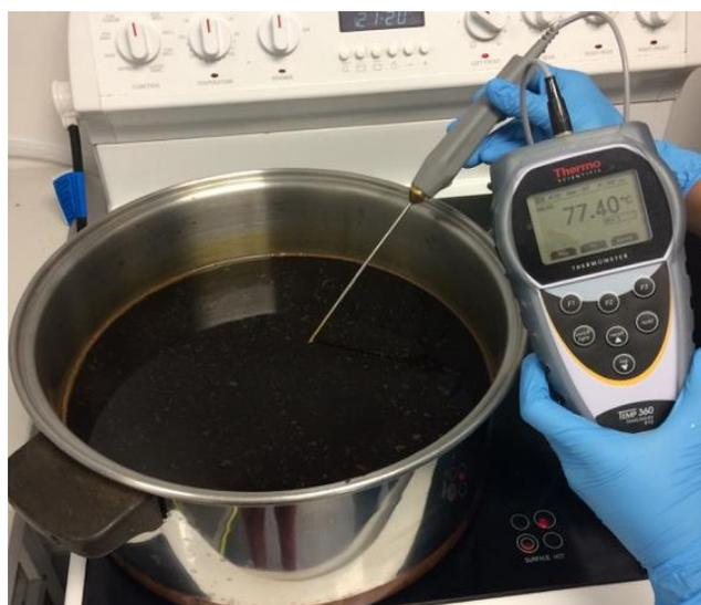
**Figure 7.** Suspension of water and molasses heated to 77.40°C.
