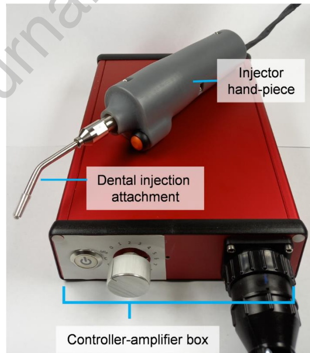
Figure 1 – Needle-free jet injector driven by an electric motor.
