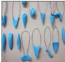
06. Range of handle Prototypes to explore ergonomic aspects
