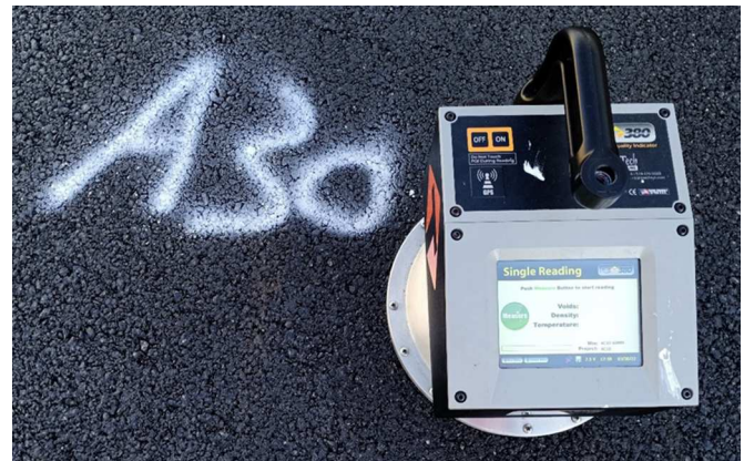
Figure 7. A PQI device measuring the density at the marked spot.
