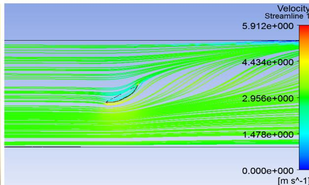
Fig 5: Flow visualization and stream lines for  $30^\circ$  tilt angle
