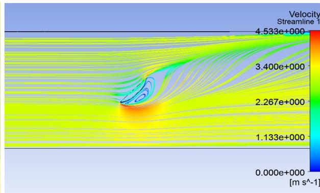
Fig 4: Flow visualization and stream lines for  $45^\circ$  tilt angle
