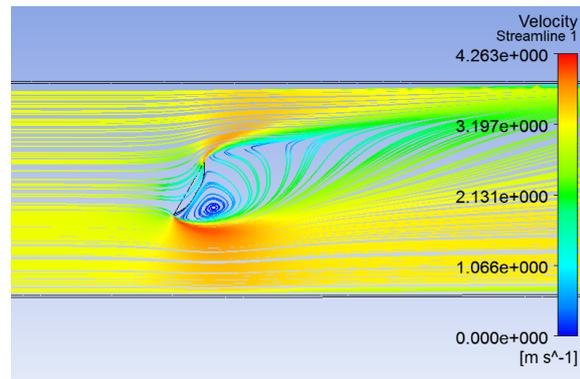
Fig 3: Flow visualization and stream lines for  $60^\circ$  tilt angle
