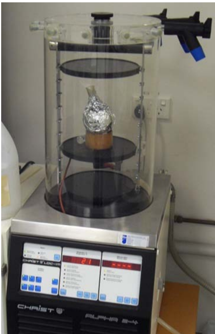
Figure 11: Freeze-drying the NZ crude fucoxanthin
