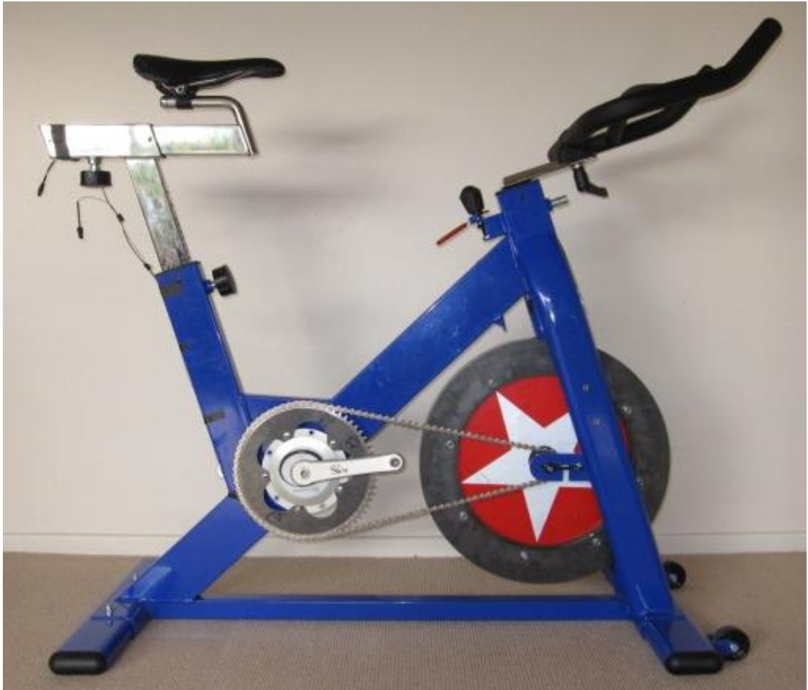
Figure 3.1. First generation inertial ergometer constructed from a stationary bicycle trainer with the stated physical properties utilised in this research.
