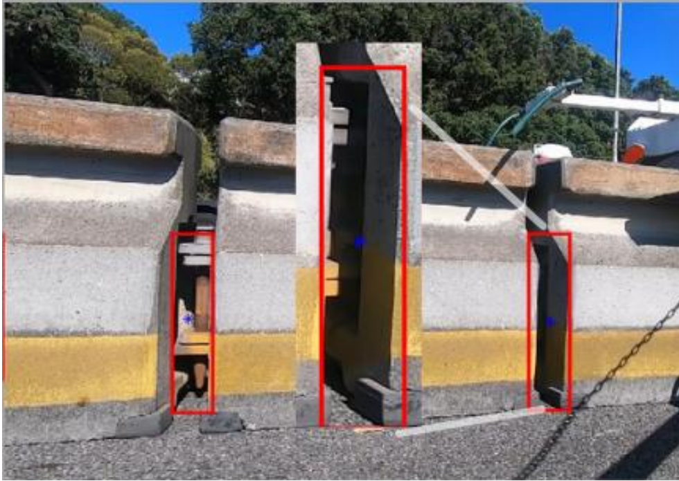
Fig. 7: ROI tracking example. Sub-section is taken out of the frame in view for further processing. Centroids are detected for all contiguous regions in the subsection before calculating the object centroid.
