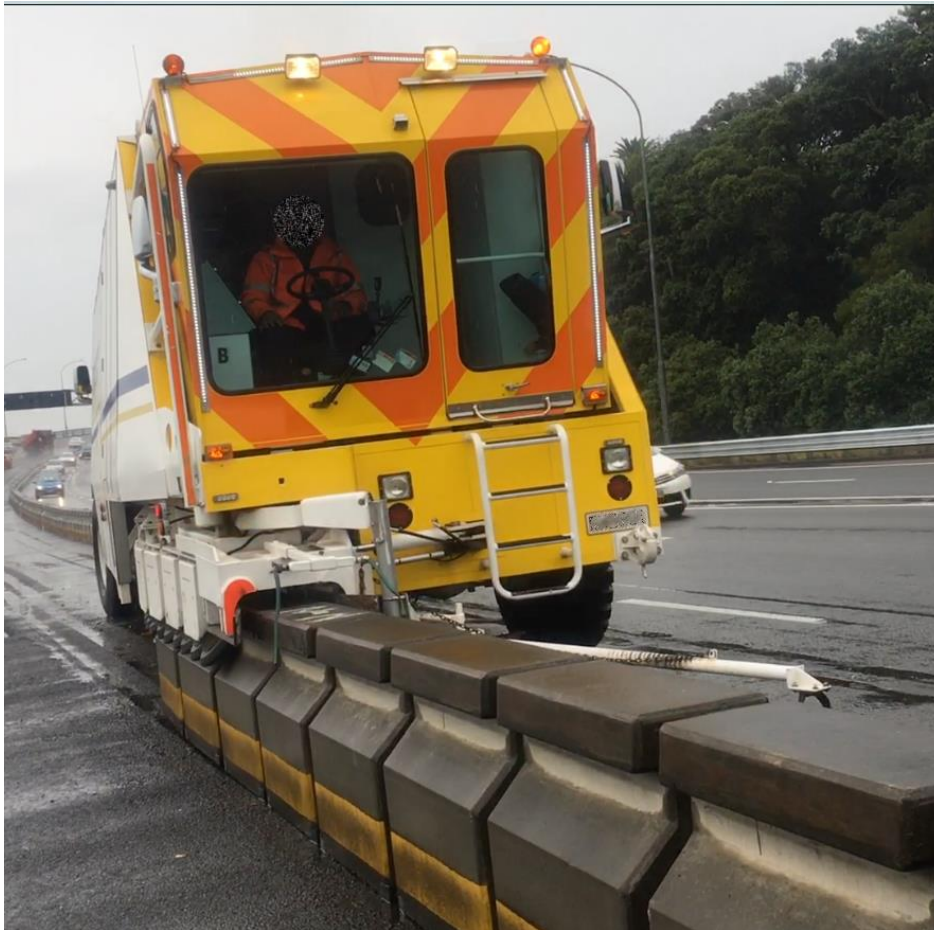
Fig. 4: The barrier transfer machine (BTM) in action. Adopted from (Bačić et al., 2020)
