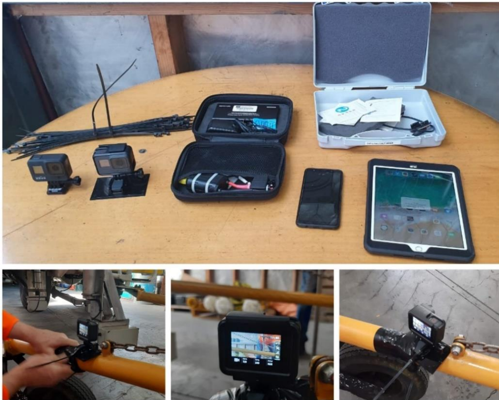
Fig. 13: Data collection setup: Samsung A7 Mobile, Apple Ipad 6, External power bank, GoPro cameras and mounting equipment, Camera mounting on BTM.
