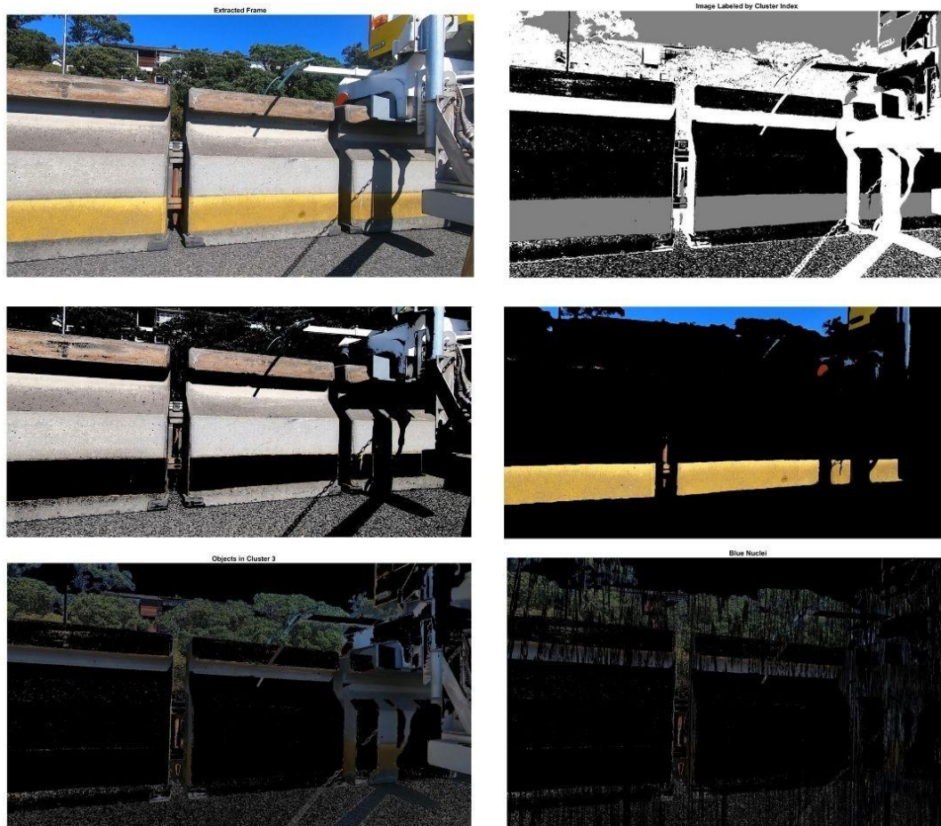
Fig. 24: Example of colour-based segmentation using K-Means clustering.
