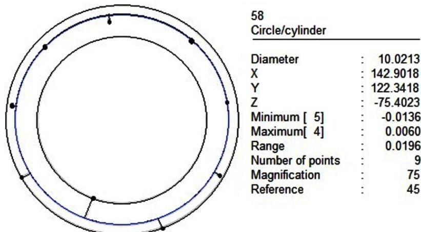
**Fig.4: A sample measurement result using CMM on experiment 16 at the top of hole with the result of maximum roundness of 0.0196**
