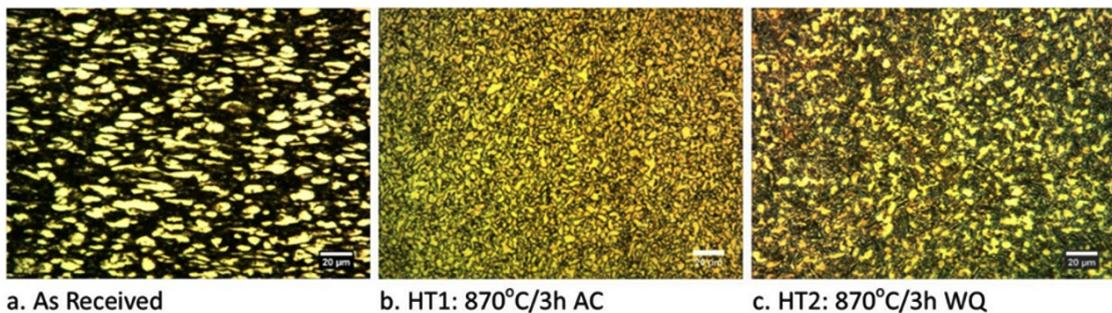
Fig. 2: Microstructure of Ti-6246 of different heat treatment: (a) as received (AR), (b) heat treated at  $870^\circ\text{C}$  for 3 hours then followed by air cooling, and (c) heat treated at  $870^\circ\text{C}$  for 3 hours followed by water quenching.
