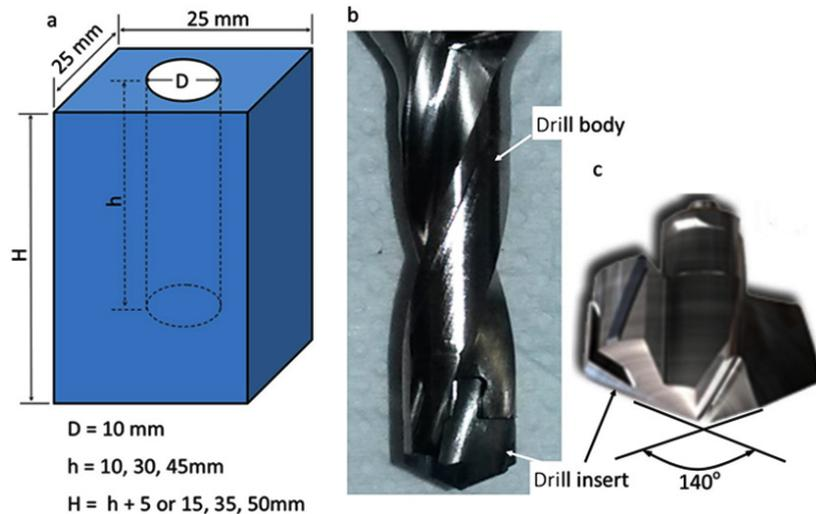
Fig. 1: Ti-6246 block dimension (a), tool set (b), and drill insert (c)
