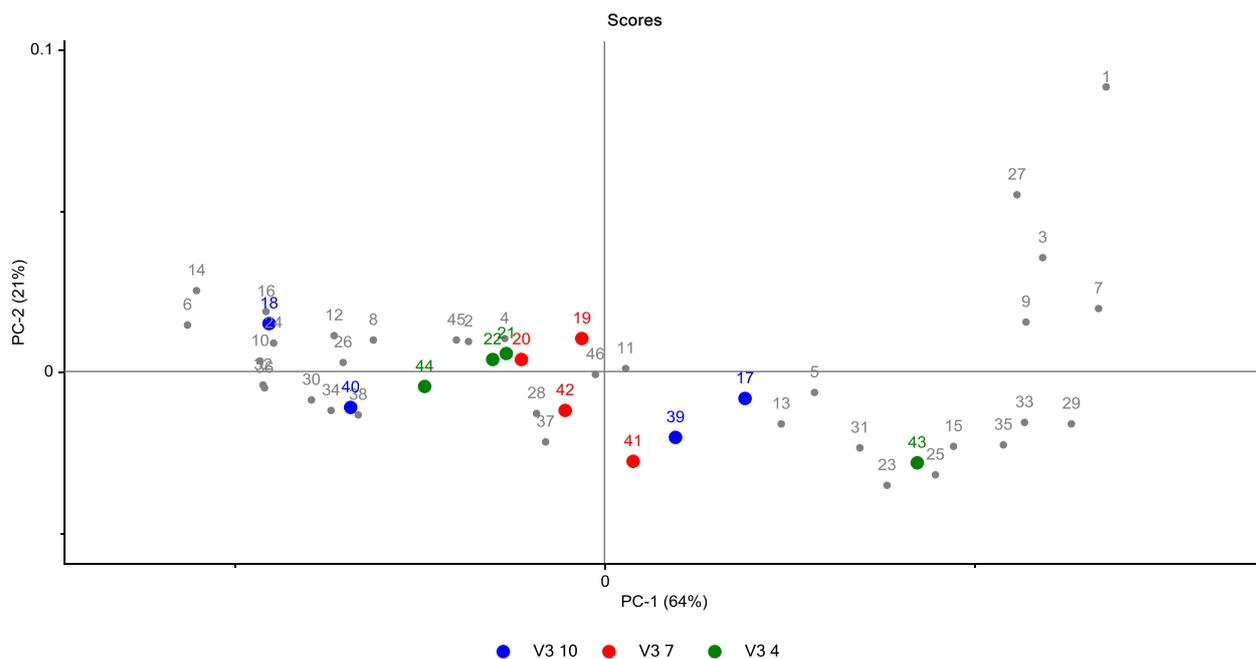
Figure 28. PCA of SEC HPLC data from the membrane separations with samples marked according to the pH of the solution during separation. The coloured samples were separated with a V3 (30 kDa MWCO) membrane at pH 10 (blue), pH 7 (red) and pH 4 (green). Remaining points (grey) are samples that were separated with uncharged membranes.
