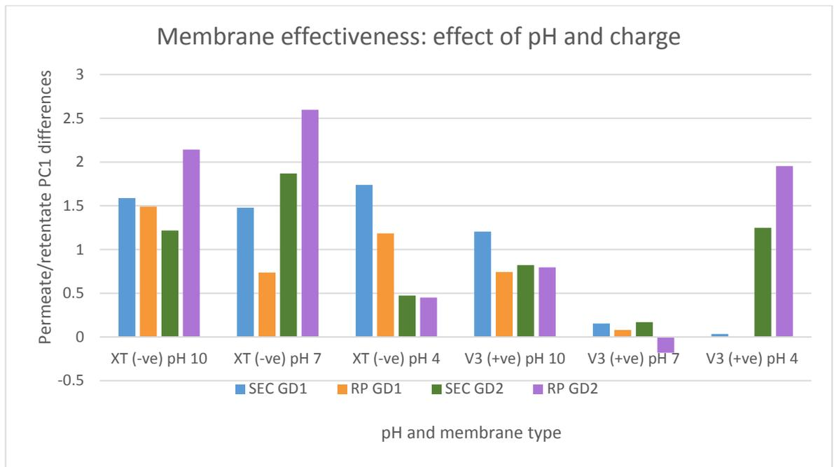
Figure 29. Effect of the membrane charge and pH of the solution on the effectiveness of the membrane separations. PC1 values from the PCA of the separations carried out at different pHs were used to calculate the effectiveness of the separations as related to charge. Retentate value subtracted from permeate value indicates the effectiveness of separation.
