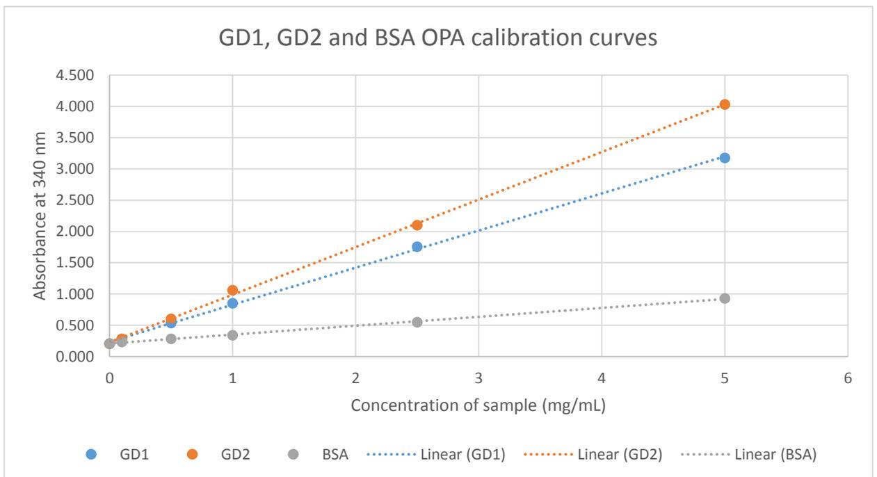
Figure 34. OPA assay standard curves for concentrations of GD1, GD2 and BSA. Note the very different slope for the BSA relative to the hydrolysates illustrating why it is not a suitable standard for these samples.
