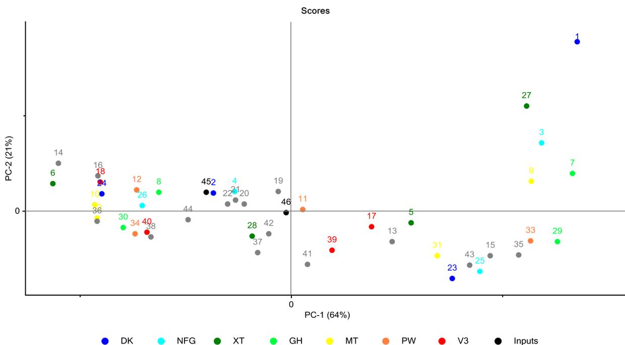
Figure 23. PCA of SEC HPLC data from the membrane separations with samples marked according to the membrane used. All coloured samples were separated at pH 10. Samples separated at pH 4 or 7 are coloured grey. MWCOs of membranes: DK 150-300 Da; NFG 600-800 Da; XT 1 kDa; GH 2.5 kDa; MT 5 kDa; PW 10 kDa; V3 30 kDa.
