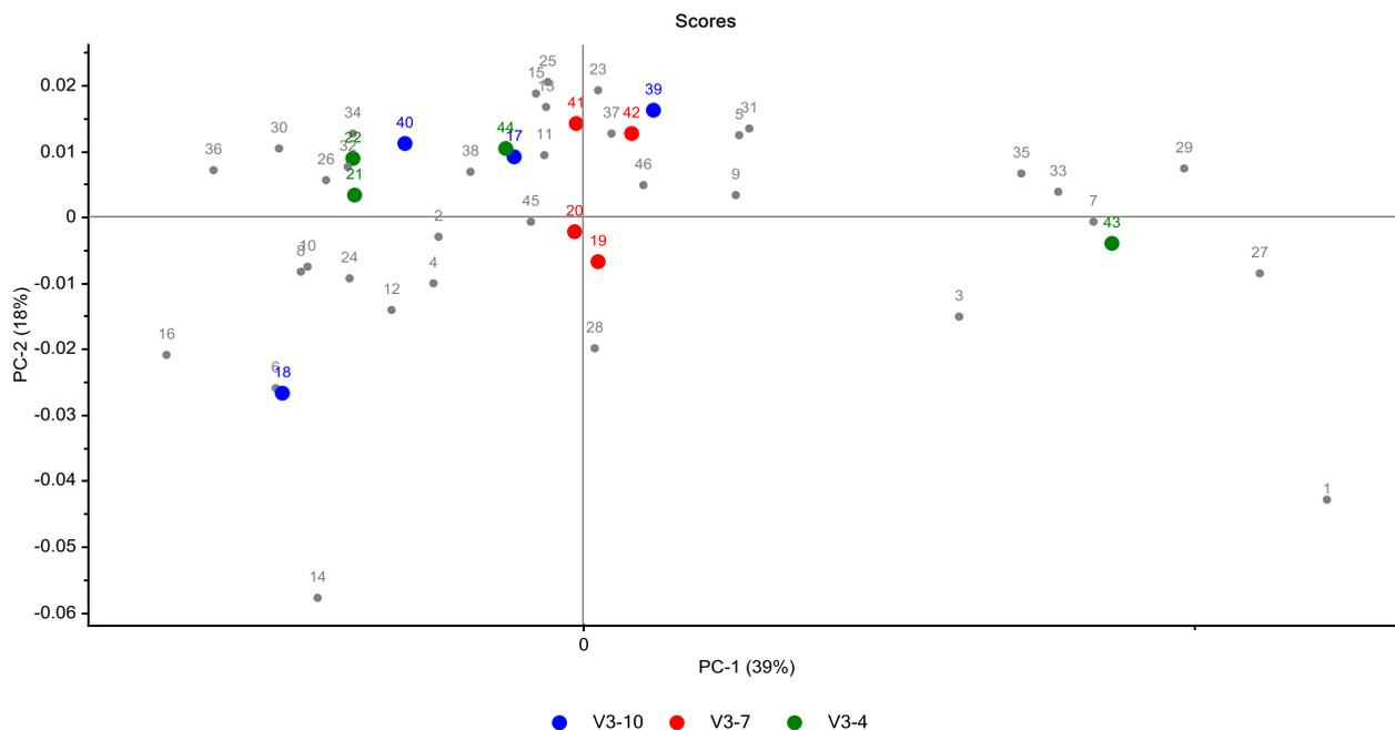
Figure 27. PCA of RP HPLC data from the membrane separations with samples marked according to the pH of the solution during separation. The coloured samples were separated with a V3 (30 kDa MWCO) membrane at pH 10 (blue), pH 7 (red) and pH 4 (green). Remaining points (grey) are samples that were separated with uncharged membranes.
