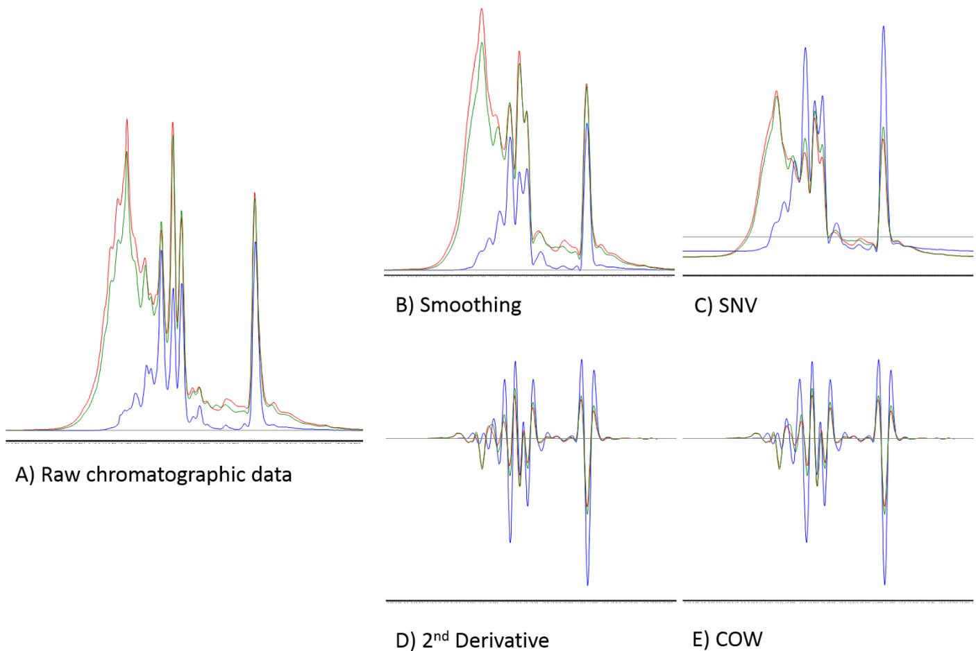
Figure 1. Effects of pre-processing transformations on the raw chromatographic data.
