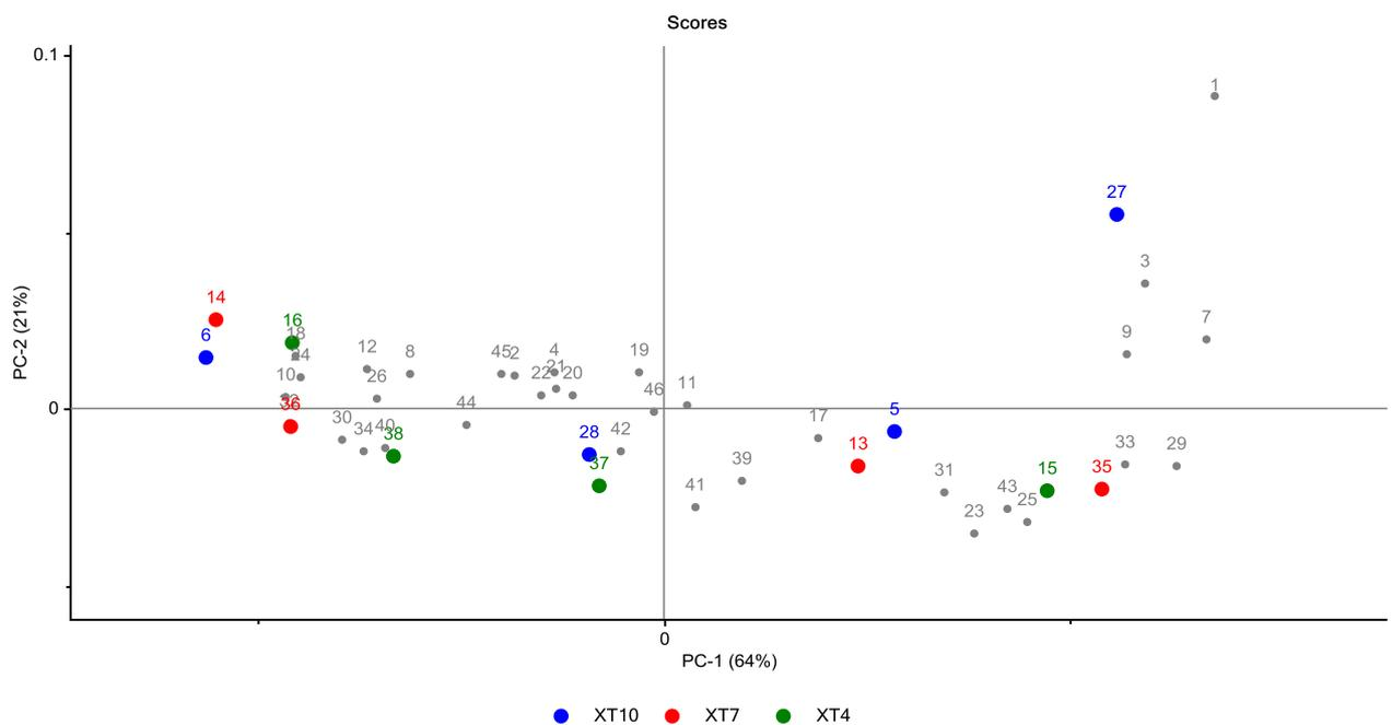
Figure 26. PCA of SEC HPLC data from the membrane separations with samples marked according to the pH of the solution during separation. The coloured samples were separated with an XT (1 kDa MWCO) membrane at pH 10 (blue), pH 7 (red) and pH 4 (green). Remaining points (grey) are samples that were separated with uncharged membranes.
