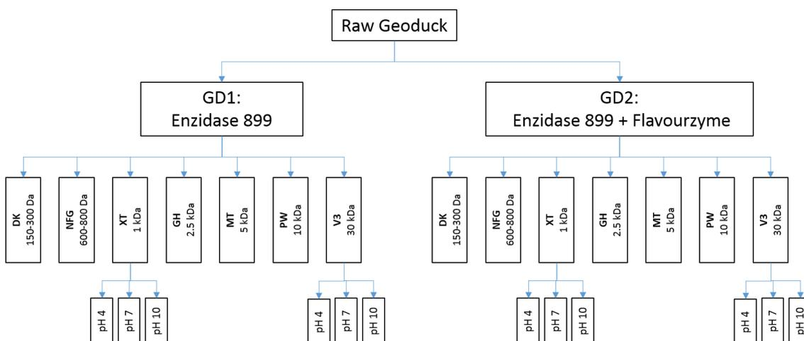
Figure 3. Experimental schematic for the membrane separations of the geoduck hydrolysates outlining the different enzyme treatments, membrane processing and pH modifications used.
