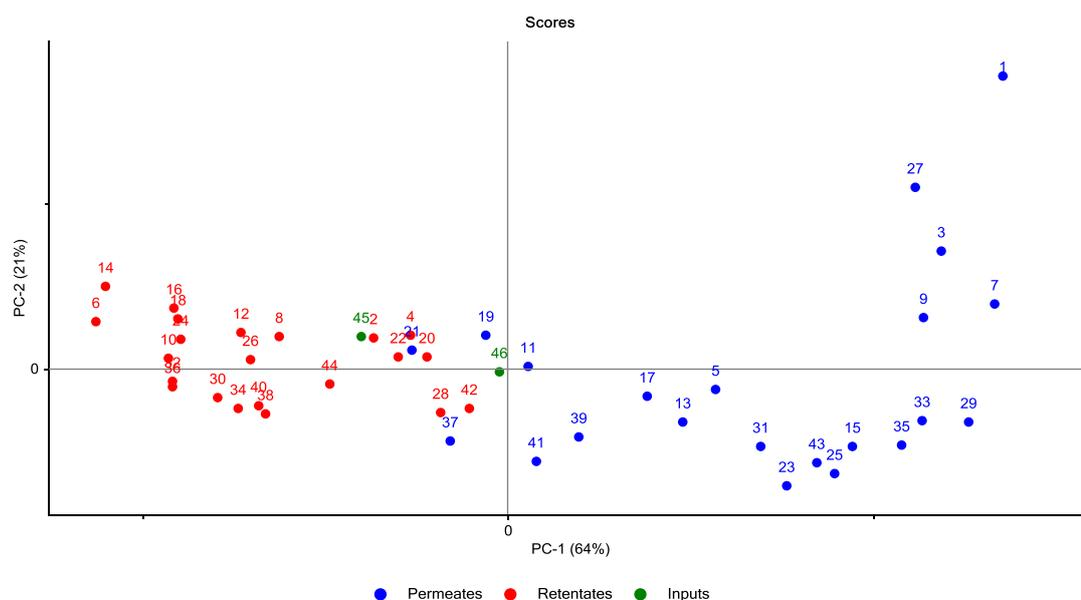
Figure 19. PCA of SEC HPLC data from the membrane separations with samples marked according to whether they are input (green), permeate (blue), or retentate (red).
