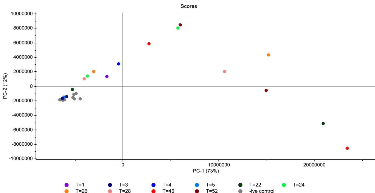
Figure 9. Principle Component Analysis (PCA) scores plot illustrating the arrangement of the samples according to time. The plot was generated from the 215 nm data of the Reverse Phase (RP) separations of the hydrolysates. Digestion times are indicated in the legend. Negative control samples are grey.
