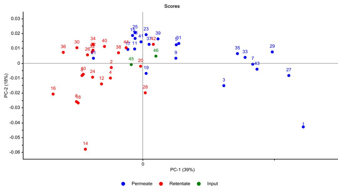
Figure 18. PCA of RP HPLC data from the membrane separations with samples marked according to whether they are input (green), permeate (blue), or retentate (red).
