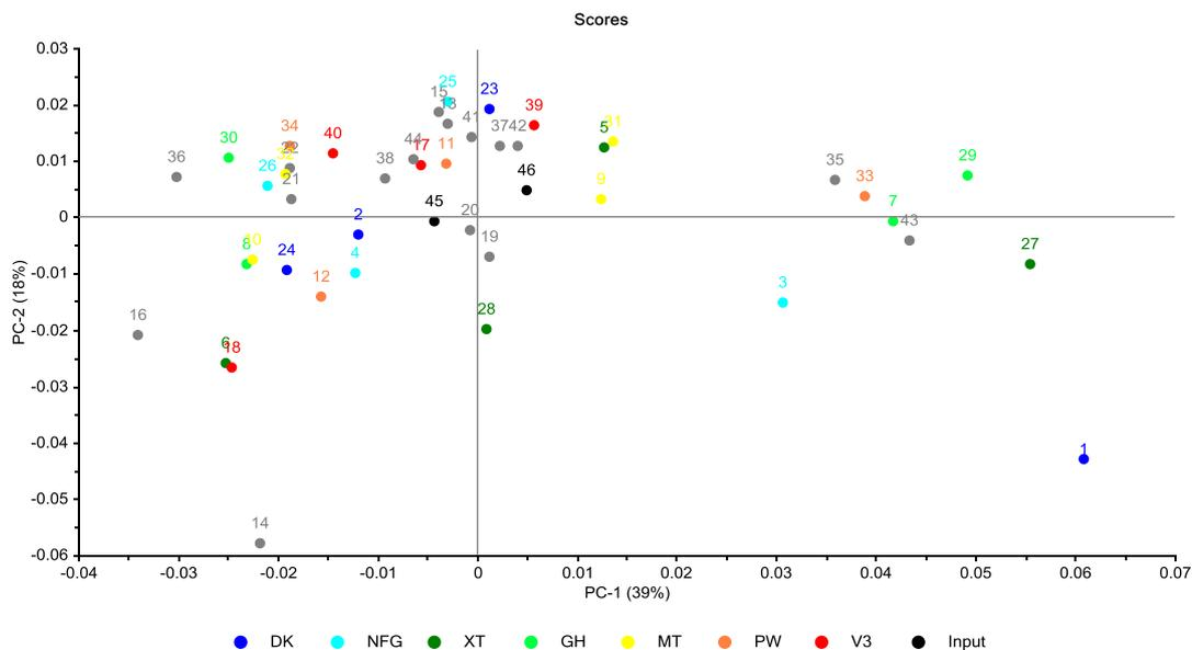
Figure 22. PCA of RP HPLC data from the membrane separations with samples marked according to the membrane used. All coloured samples were separated at pH 10. Samples separated at pH 4 or 7 are coloured grey. MWCOs of membranes: DK 150-300 Da; NFG 600-800 Da; XT 1 kDa; GH 2.5 kDa; MT 5 kDa; PW 10 kDa; V3 30 kDa.
