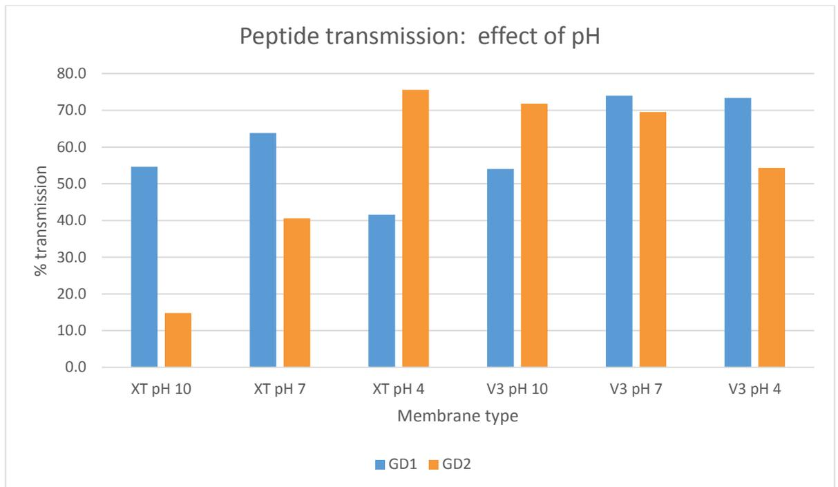
Figure 15. Effect of pH on peptide transmission through two membranes (XT membrane: 1 kDa MWCO, -ve charge. V3 membrane: 30 kDa MWCO, +ve charge).
