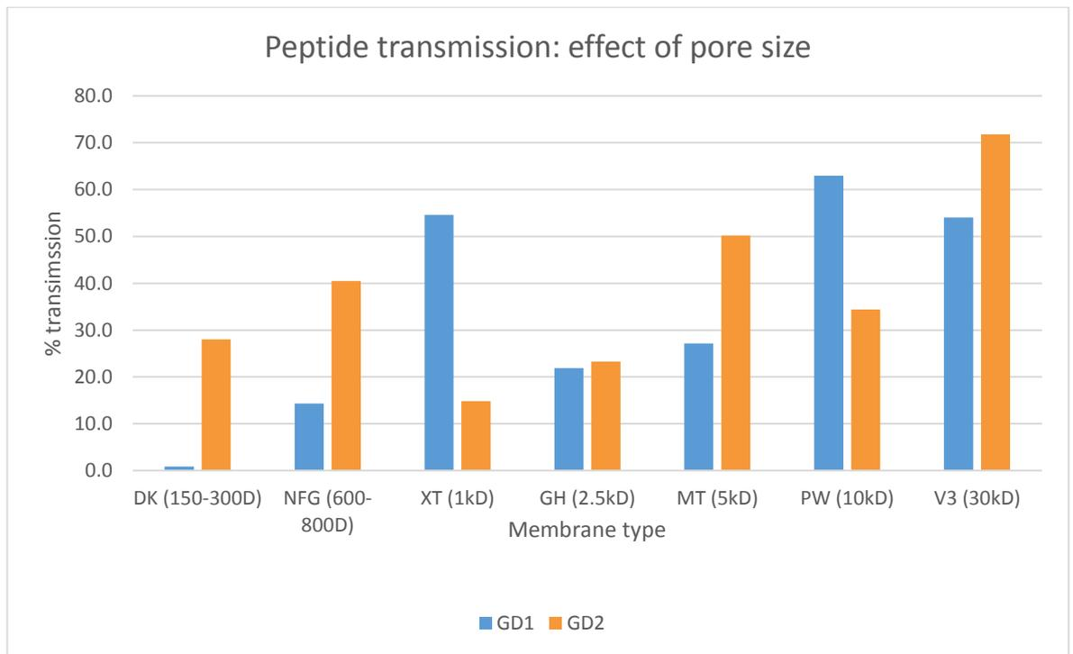
Figure 14. Effect of pore size on peptide transmission through membranes with differing pore size characteristics.
