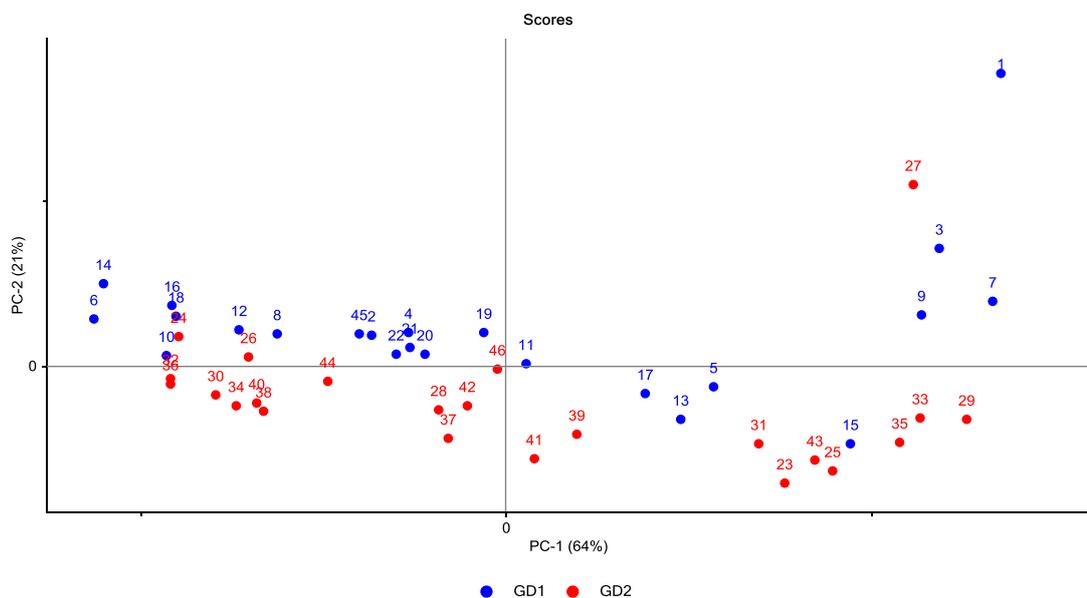
Figure 21. PCA of SEC HPLC data from the membrane separations with samples marked according to the enzyme treatment. GD1/ Enzidase 899 (blue) and GD2/ Enzidase 899+flavourzyme (red).
