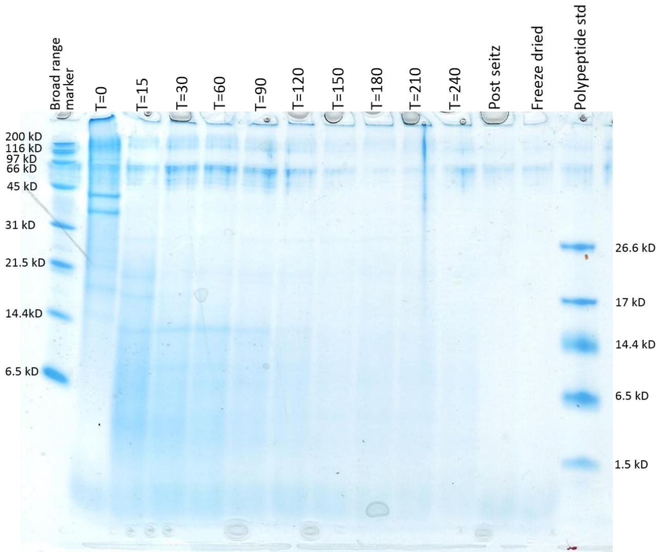
Figure 12. 16.5% PAGE gel of geoduck hydrolysis at various times with Enzidase 899 (GD1).
