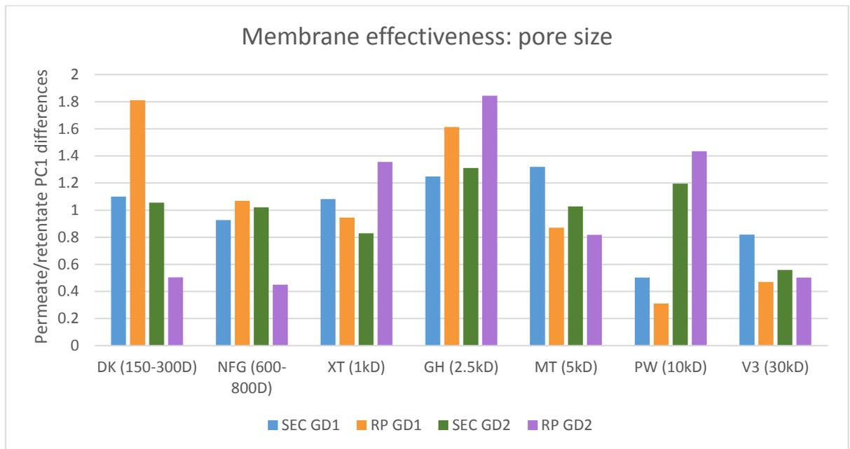
Figure 24. Membrane effectiveness as related to membrane MWCO. The difference between the PC1 scores of the permeate and retentate samples is indicative of the effectiveness of the separation. Membrane separations are all from the experiments performed at pH 10. Data is arranged by chromatography mode used and hydrolysate type: SEC of GD1 (blue), RP of GD1 (orange), SEC of GD2 (green) RP of GD2 (purple).
