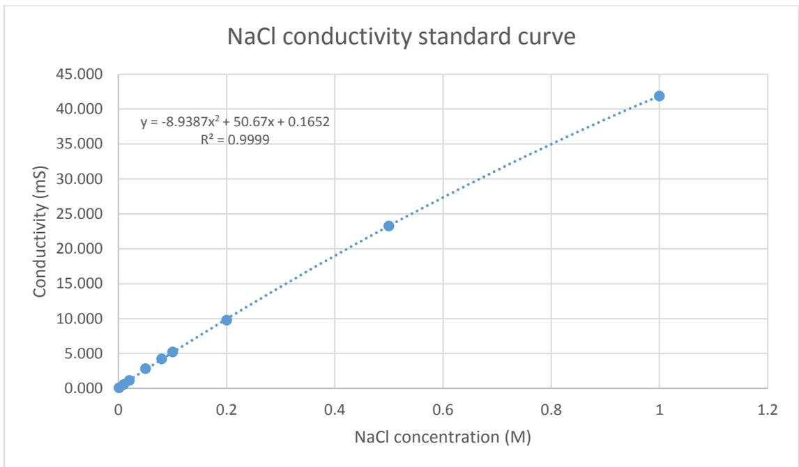
Figure 33. NaCl conductivity standard curve.
