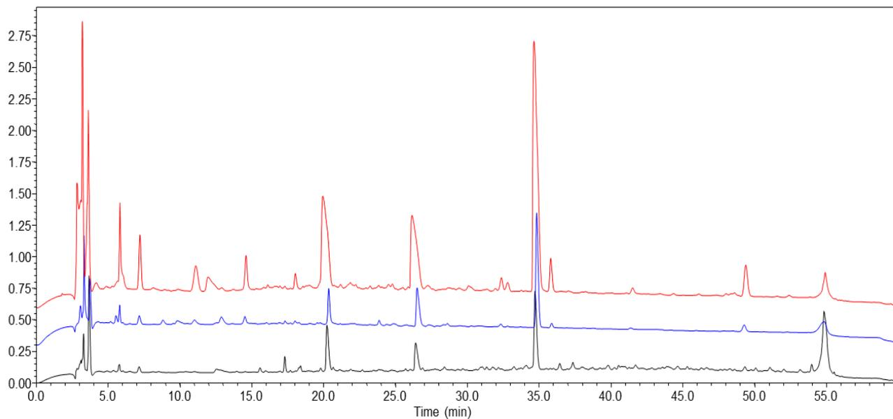
Figure 7. Overlays of 215 nm HPLC traces from geoduck digest time points after 1 hour (black), 22 h (blue) and 52 h (red). Samples were separated on a Phenosphere Next C18 reverse phase (RP) column. Buffer A was 0.1%TFA and buffer B was acetonitrile. The samples were loaded in 0% B and held for 5 min and then the gradient was increased to 25% B over 45 min. The concentration of B was increased to 40% B for 5 min and then run at 0% B for 5 min.
