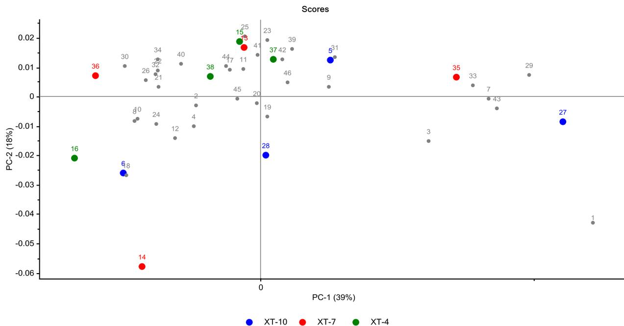
Figure 25. PCA of RP HPLC data from the membrane separations with samples marked according to the pH of the solution during separation. The coloured samples were separated with an XT (1 kDa MWCO) membrane at pH 10 (blue), pH 7 (red) and pH 4 (green). Remaining points (grey) are samples that were separated with uncharged membranes.
