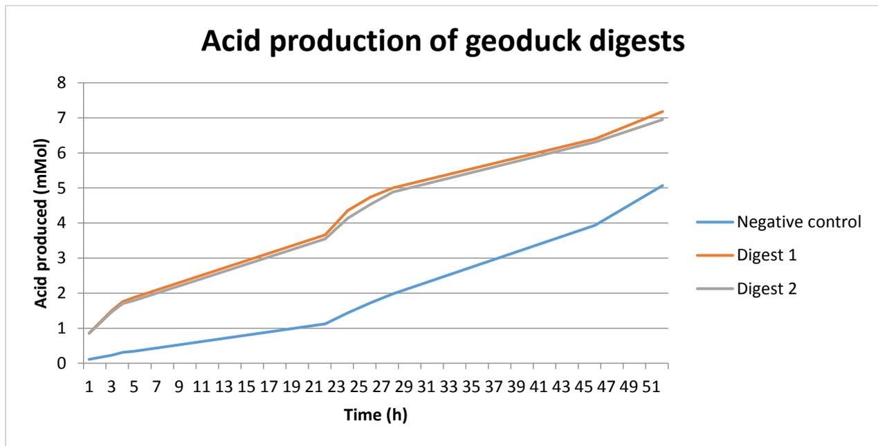
Figure 5. Acid produced by protein hydrolysis of geoduck tissue over 52 h as determined by NaOH titration. Negative control (blue) contains geoduck tissue with no added protease. Digest 1 (red) and digest 2 (green) are replicate samples containing 0.5% (w/v) Enzidase 899 and flavourzyme.
