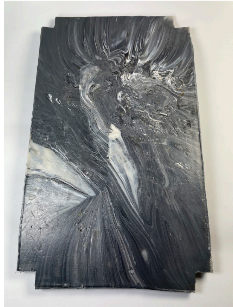
Figure 29 & 30: 600 mm x 350 mm flat HDPE sheet material.
