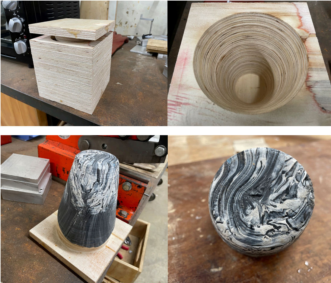
Figure 34: Cone shape compression moulding
