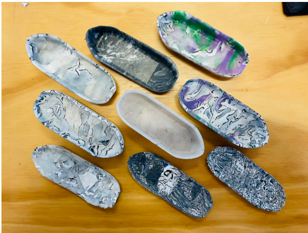
Figure 31: Compression moulding of HDPE using a latex mould
