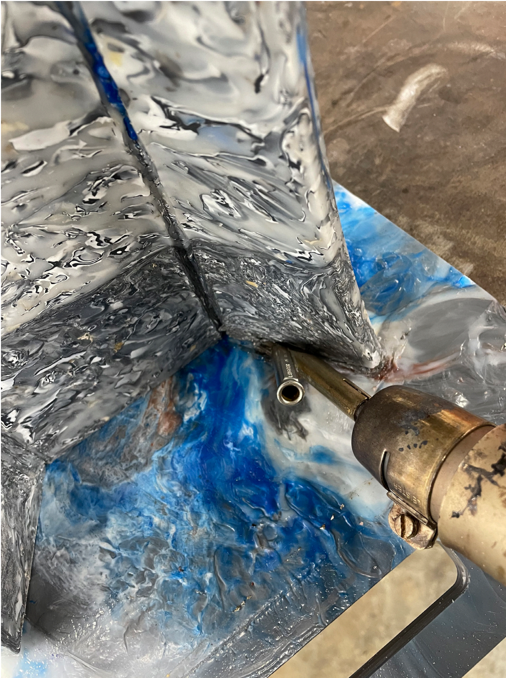
Figure 70: Stool top welding
